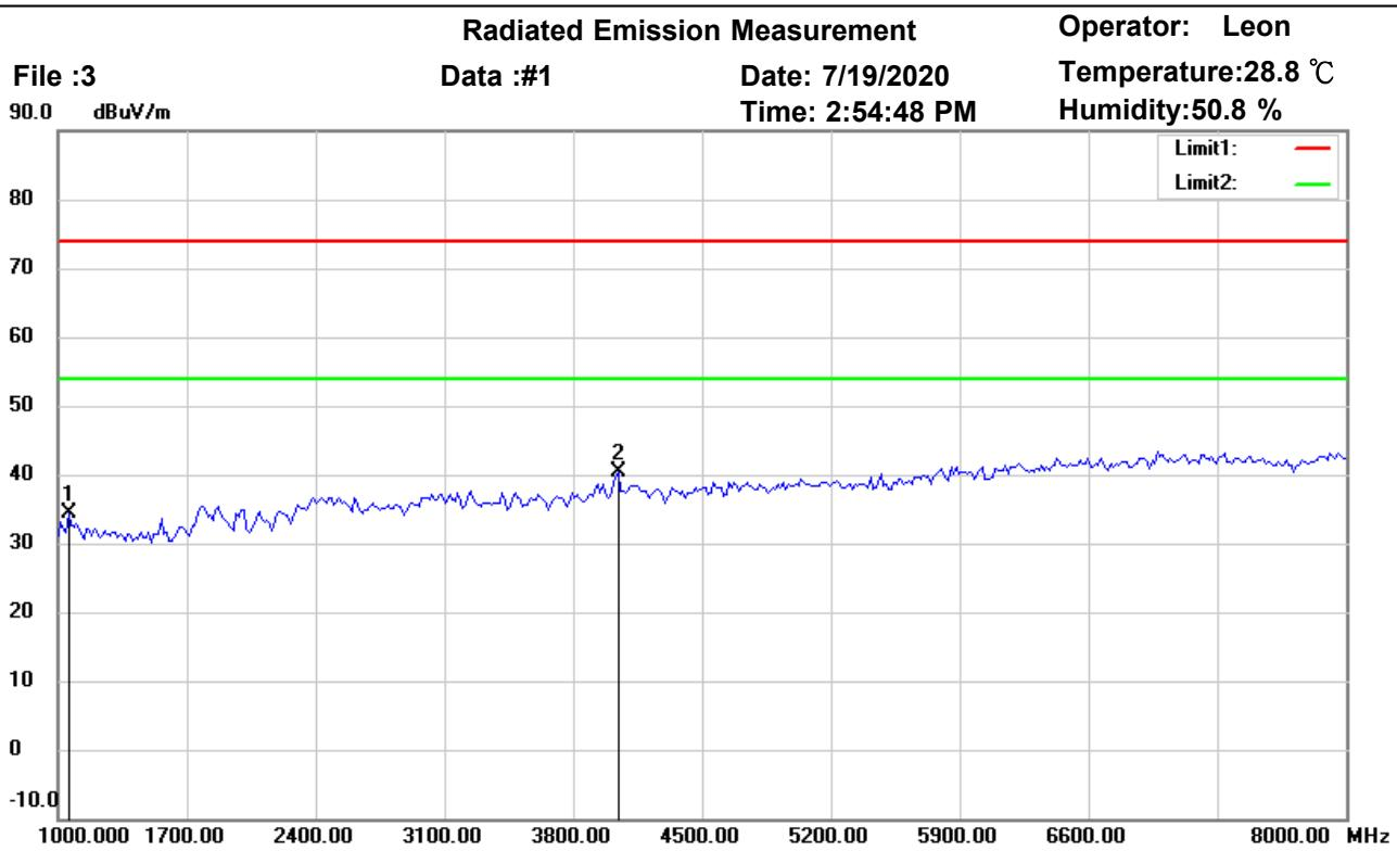
**Site :** Chamber**Condition :** FCC\_part 15 RE-Class B\_Above 1GHz\_PK**Polarization:** *Horizontal***EUT :** W6M22005-19938**Power :** 120 V.a.c.**M/N:****Distance:** 3m**Test Mode :** RX 802.11n20 CH1**Note :**
