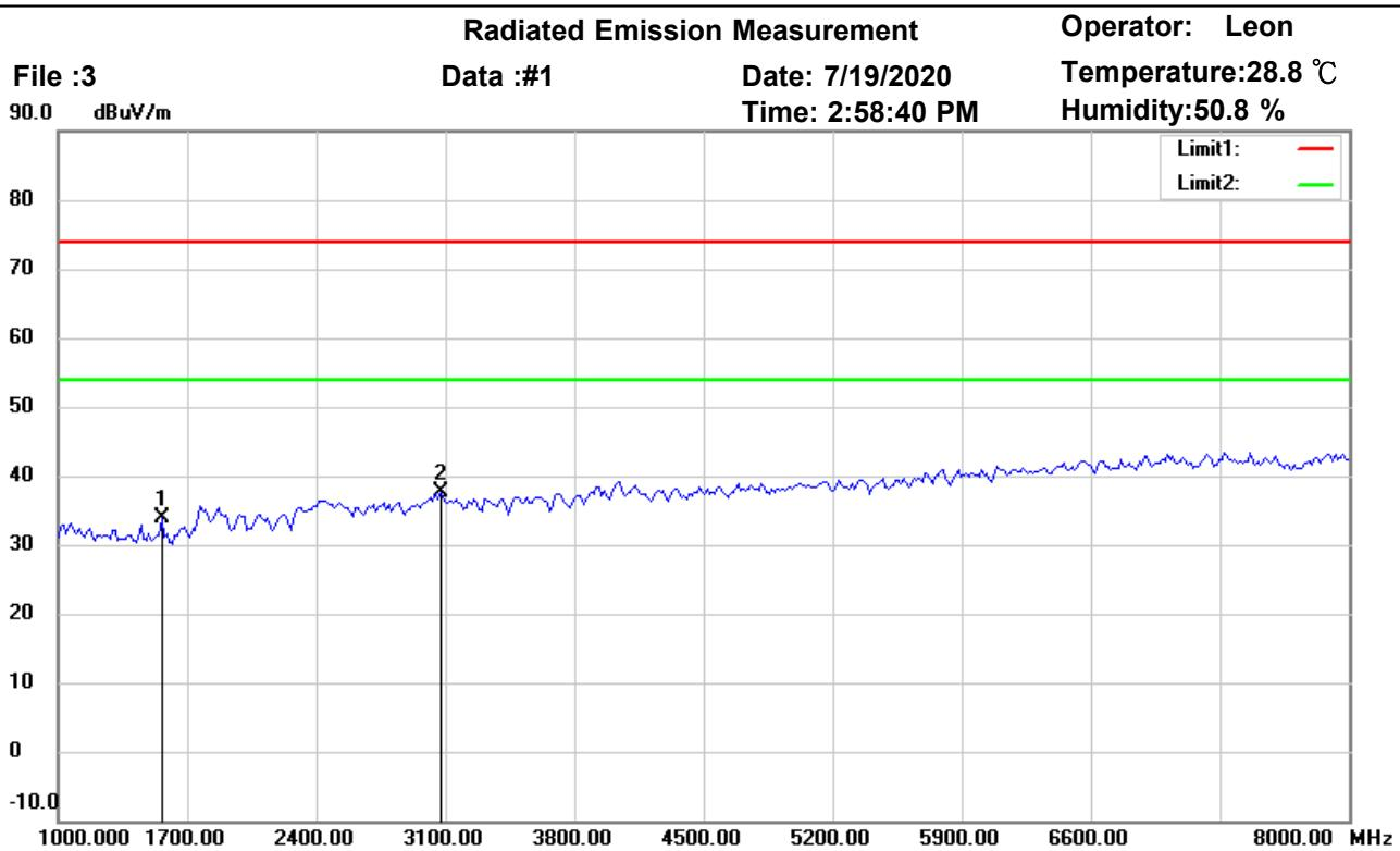
**Site :** Chamber**Condition :** FCC\_part 15 RE-Class B\_Above 1GHz\_PK**Polarization:** *Horizontal***EUT :** W6M22005-19938**Power :** 120 V.a.c.**M/N:****Distance:** 3m**Test Mode :** RX 802.11n40 CH1**Note :**
