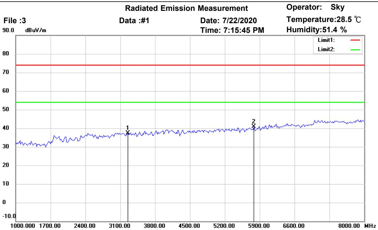
**Site :** Chamber**Condition :** FCC\_part 15 RE-Class B\_Above 1GHz\_PK**Polarization:** *Horizontal***EUT :** W6M22005-19938**Power :** 120 V.a.c.**M/N:****Distance:** 3m**Test Mode :** RX 802.11ac CH42**Note :**
