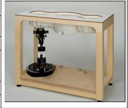
The shell corresponds to the specifications of the Specific Anthropomorphic Mannequin (SAM) phantom defined in IEEE 1528 and IEC 62209-1. It enables the dosimetric evaluation of left and right hand phone usage as well as body mounted usage at the flat phantom region. A cover prevents evaporation of the liquid. Reference markings on the phantom allow the complete setup of all predefined phantom positions and measurement grids by teaching three points with the robot.
