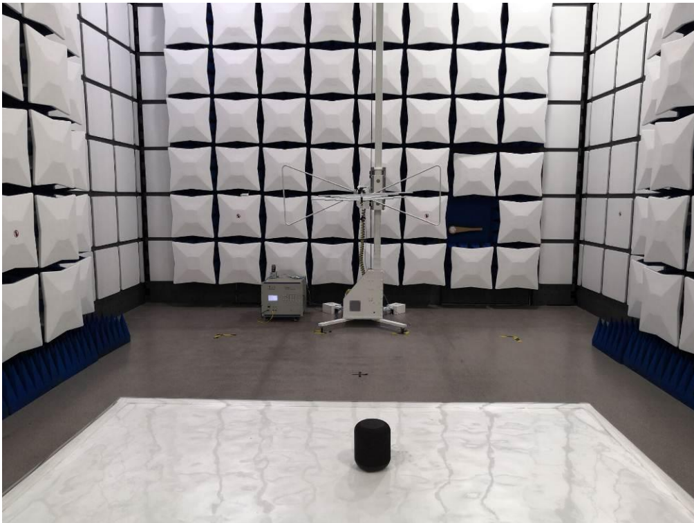
FCC RADIATED EMISSION TEST SETUP
