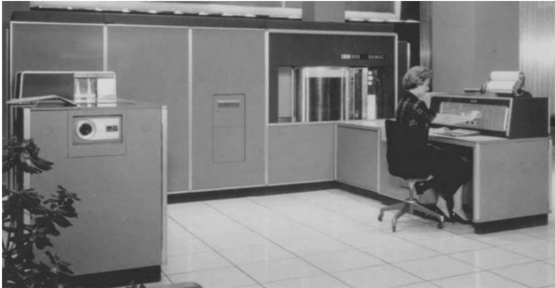
FIGURE E5.17.6 The RAMAC disk drive from IBM, made in 1956, was the first disk drive with a moving head and the first with multiple platters. The IBM storage technology Web site has a discussion of IBM's major contributions to storage technology.
