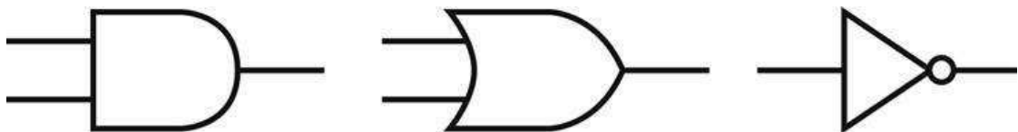
FIGURE A.2.1 Standard drawing for an AND gate, OR gate, and an inverter, shown from left to right. The signals to the left of each symbol are the inputs, while the output appears on the right. The AND and OR gates both have two inputs. Inverters have a single input.
