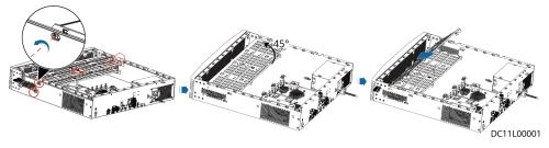
3. Place the hard disks with ports facing upwards and align the screw holes on the hard disk tray with the hard disks and fasten the screws. Before the installation, ensure that the fastener of the hard disk tray is on a different side from the hard disk port, as shown in the lower left figure.
