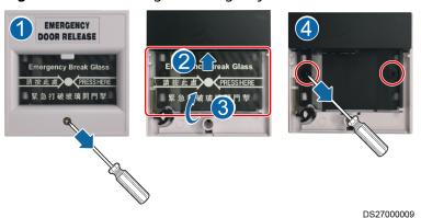
**Step 2** Install a new emergency door release button.
