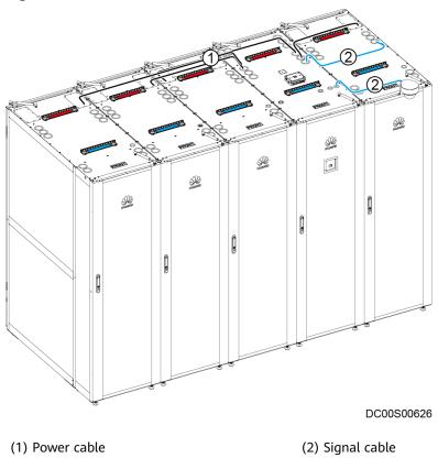
The Converged Cabinet fitting bag contains 70 plastic cable ties that can be installed on holes at the top of the cabinet for binding cables, as shown in **Figure 4-187**.
