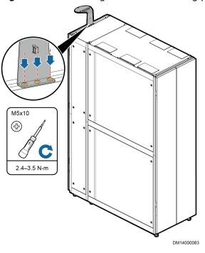
Figure 4-123 Installing a camera mounting plate
