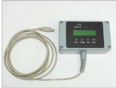
[1] Right: External control panel.
