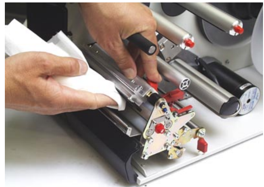
Fig. 1 Cleaning of the printhead – the printhead needs not to be unplugged (Fig: Dispenser version).
