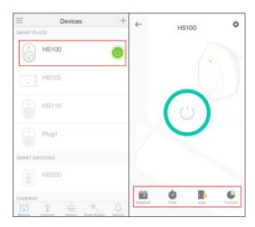
9. Tap to enter the interface of Device Settings, click on "Name and Icon" can edit the name and icon of the smart plug, click on "Device Info" can view the basic information of the smart plug.
