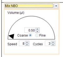
Sets the mixing volume and speed without a blowout after the dispense.
