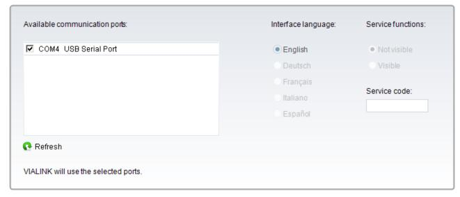
VIALINK will check the selected COM ports if a Programming Stand or instrument (VIAFLO 96/384/ASSIST) is connected.
