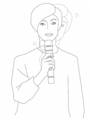
Figure 1-4 How to hold the microphone when using the "Near" setting
