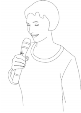
Figure 1-5 Optimum speaking distance when the ALC function is deactivated
