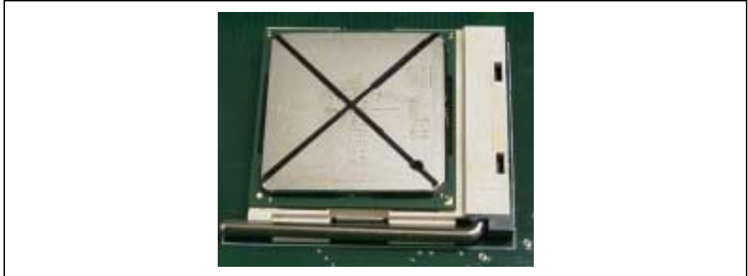
Figure 4. Desired Thermocouple Location
