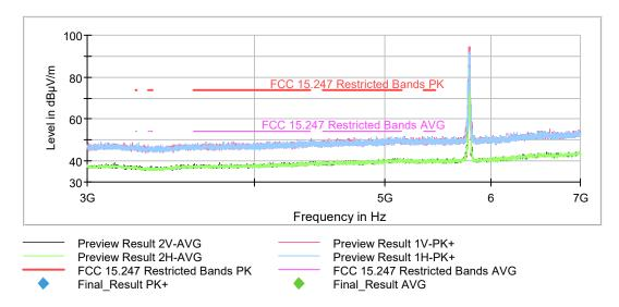
The peak above the limit is the WLAN 5 GHz carrier frequency (5785 MHz).
