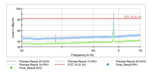
The peak above the limit is the WLAN 5 GHz carrier frequency (5785 MHz).
