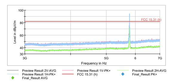
The peak above the limit on the right is the WLAN 5 GHz carrier frequency (5785 MHz).
