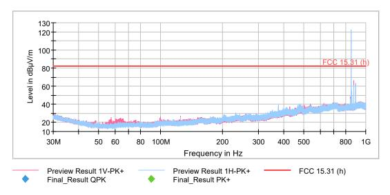
The peak above the limit is the 2G 850 carrier frequency (848.8 MHz).
