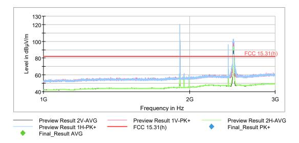
The peak above the limit on the left is the 2G 1900 carrier frequency (1909.8 MHz).
