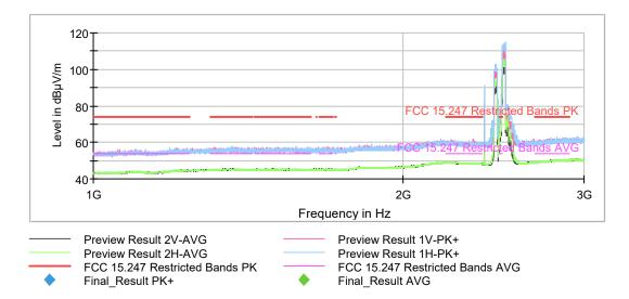
The peak above the limit on the left is the BT EDR carrier frequency (2402 MHz).
