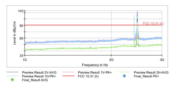
The peak above the limit on the left is the BT EDR carrier frequency (2402 MHz).
