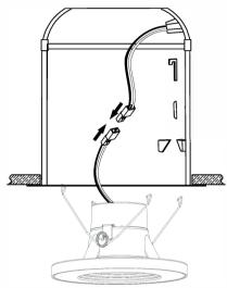
Insert the torsion springs into the fixture housing brackets. Gently push the product up and torsion springs so they begin to expand and lift the product in place.
