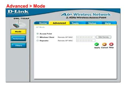
The DWL-700AP can be configured to perform in any one of three modes, as a wireless access point, as a wireless client, or as a wireless repeater.
