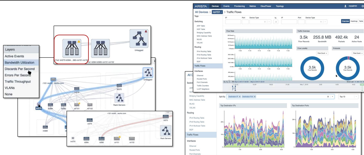
Figure 12. Network Visibility via the CloudVision from Device and Flow Monitoring Level
