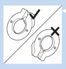
Note: Make sure that the ring of the wall mounting bracket slants downward when you hold it to the wall. If the ring of the wall mounting bracket slants upward, turn the wall mounting bracket the other way around so that it is in the correct position.
