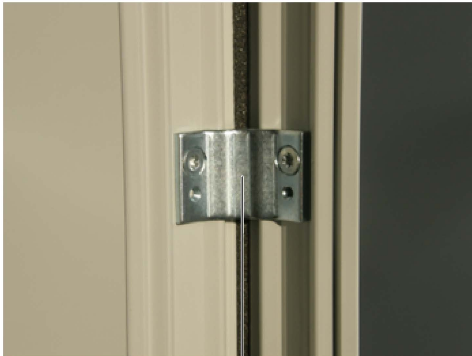
Outer cabinet connector Tightening torque: 9 Nm
