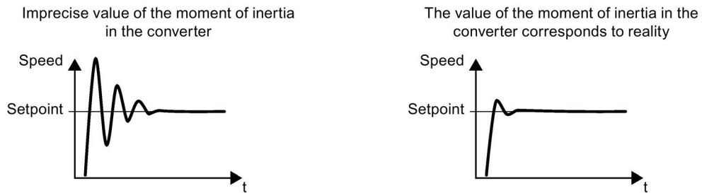
Figure 9-27 Influence of the moment of inertia estimator on the speed
