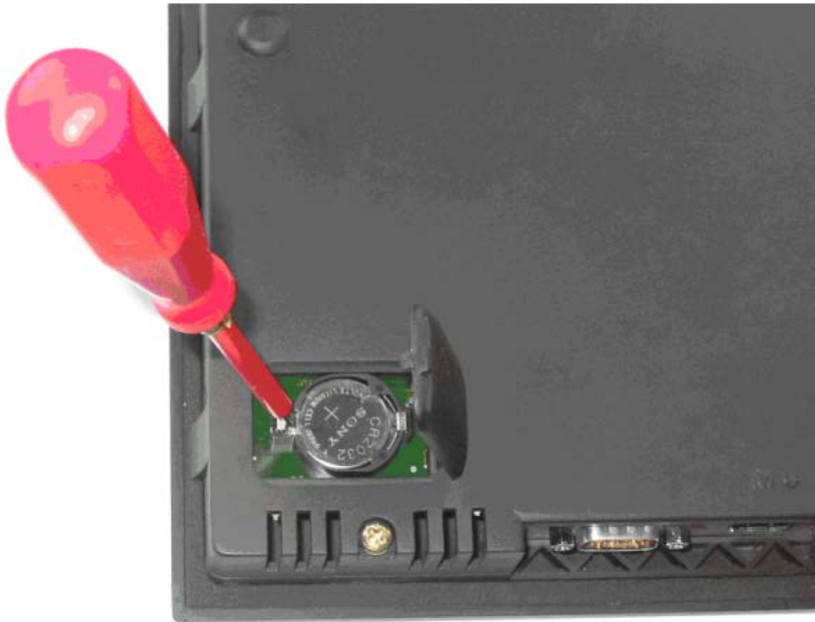
Figure 11-27 Replacing the backup battery for the cabinet operator panel
