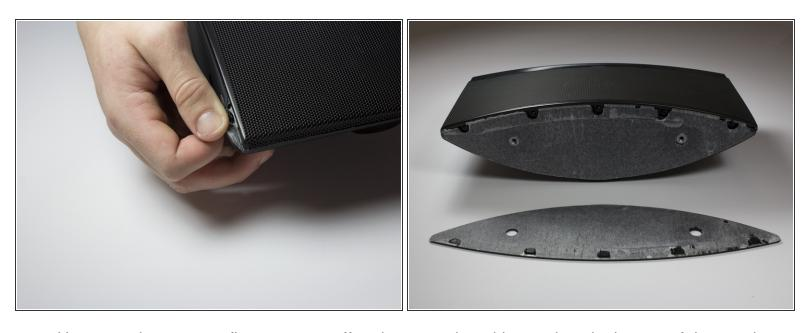
• Use a spudger or your fingers to pry off and remove the rubber pad on the bottom of the speaker.
