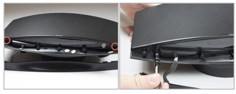
• Use a TR 10 screwdriver to remove two of the 10mm screws that secure the speaker grille.
