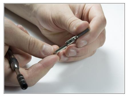
Use a 5 mm hex driver to extend the TR 10 driver. This allows the driver to access screws with deeper countersinks.
