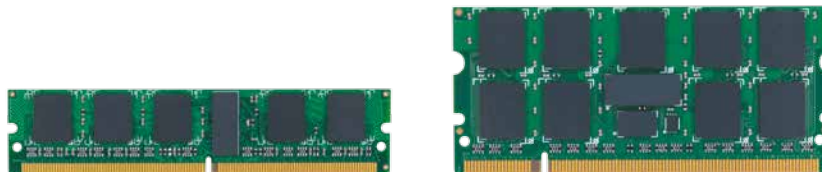
VLP MINIRDIMM WITH ECC, REGISTERED SO-RDIMM WITH ECC
