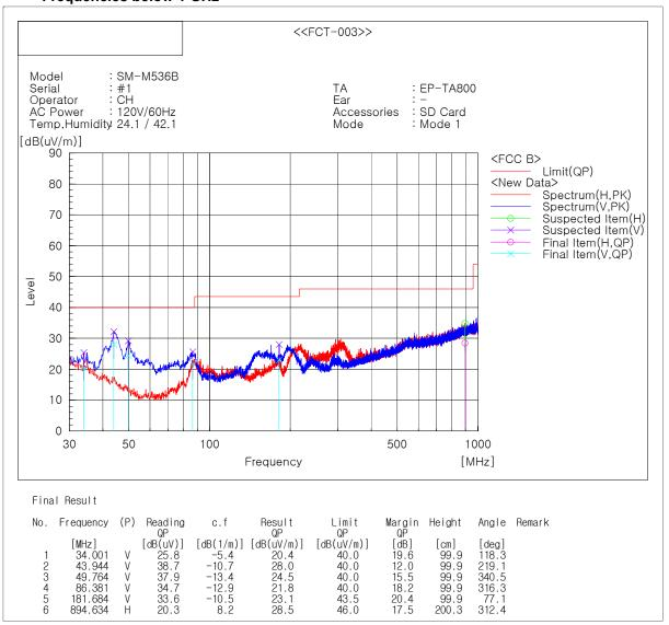
Note1) Receiving antenna polarization: Horizontal, Vertical
