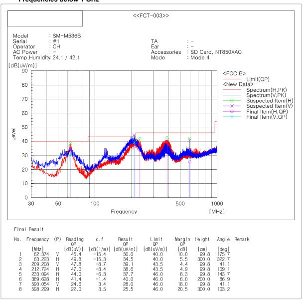
Note1) Receiving antenna polarization : Horizontal, Vertical
