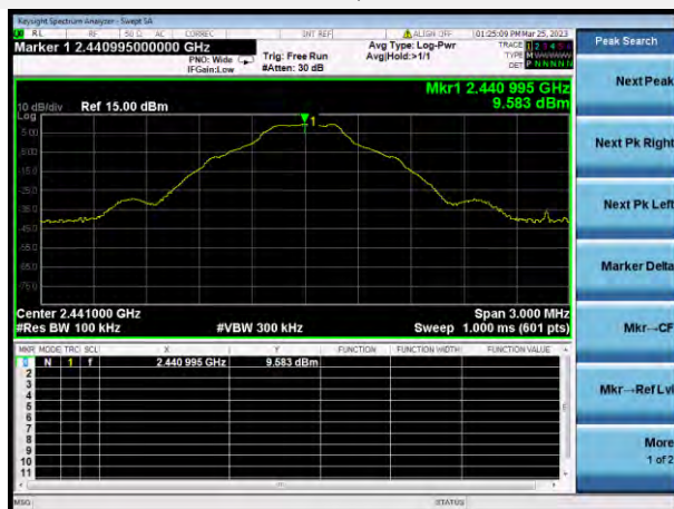
GFSK MIDDLE CHANNEL, CARRIER LEVEL
