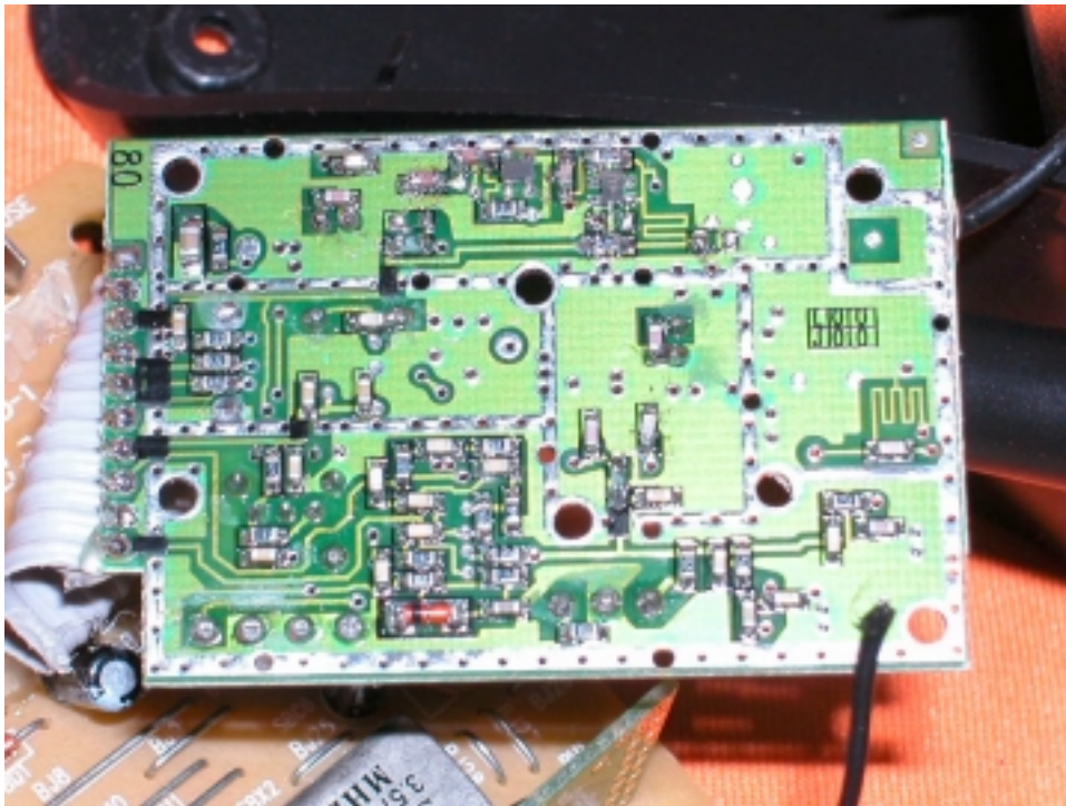
Base Oscillator PCB solder side
