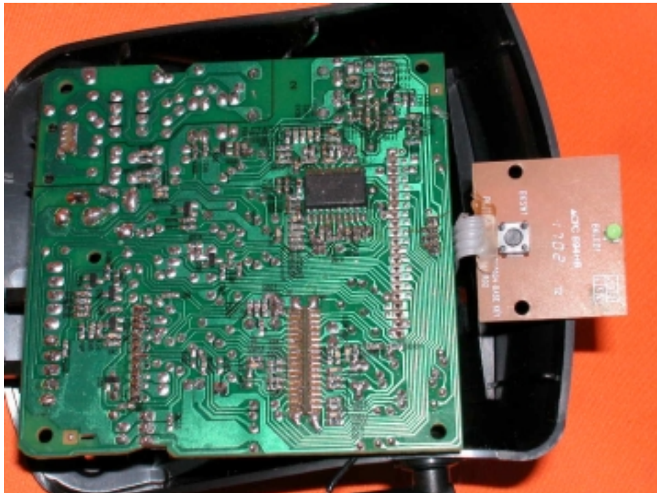
Base Main PCB solder side
