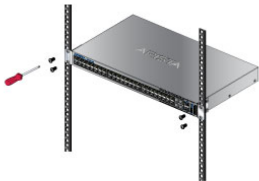
Figure 3-3: Inserting the Switch into the Rack
