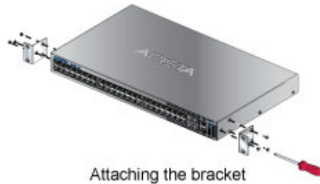
Figure 3-2: Bracket Mount Attachment to Switch
