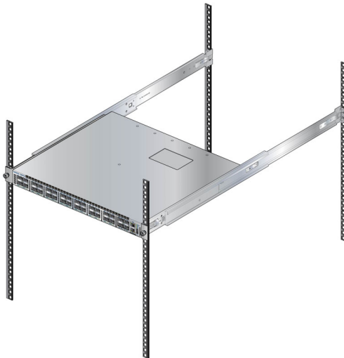
Figure 3-12: Attaching the Switch to the Rack Posts
