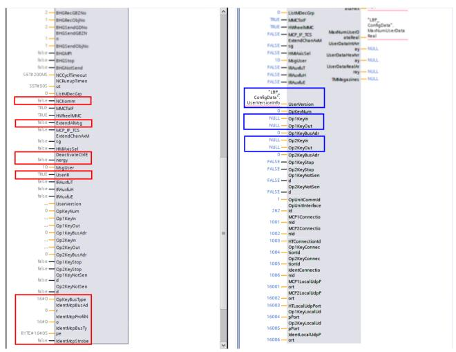
Figure A-2 Comparison of FB1 SINUMERIK 840D sl (left) and FC1 SINUMERIK ONE (right)
