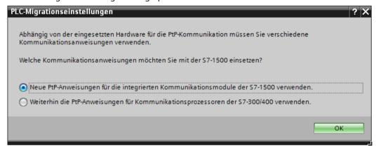
4. Select whether S7-300-PtP program blocks should be replaced automatically by the appropriate new S7-1500 operations and confirm with "OK".
