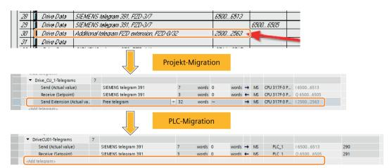
Figure 8-2 Additional telegram after project and PLC migration of a STEP 7 Classic project
