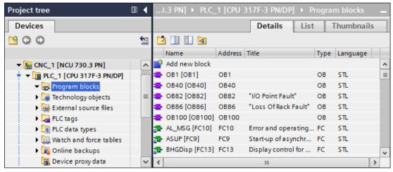
Figure 7-2 Detailed view of the basic program blocks
