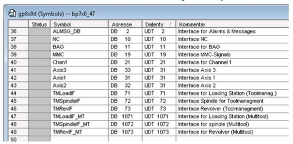
• In the TIA Portal, symbolic names (and the associated PLC data types) are defined directly in the properties of the associated blocks. For this purpose, the associated block must exist in the project.
