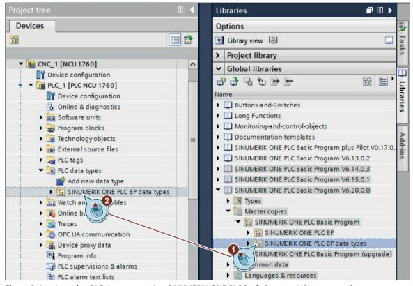
Figure 8-4 Inserting PLC data types using SINUMERIK ONE PLC Basic Program V6.x as example
