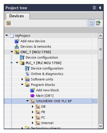
You can now check the copied blocks and manually delete the SINUMERIK PLC basic program blocks that you do not require (e.g. superfluous axis DB, channel DB, FB or FC).
