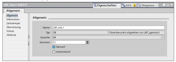
Consequently, add all required interface DBs for axes, channels, mode groups, NC, HMI and tool management as global DB to the project.
