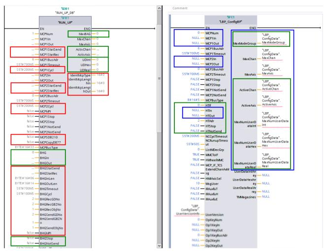
Figure A-1 Comparison of FB1 SINUMERIK 840D sl (left) and FC1 SINUMERIK ONE (right)
