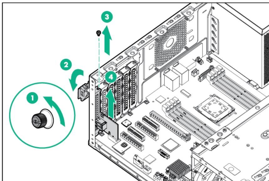
To replace the component, reverse the removal procedure. After installing the new dedicated iLO management module, enable the dedicated iLO connector ("Enabling the dedicated iLO management module" on page 59).
