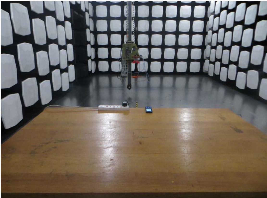
5. Part 15B Radiated emission (USB) above 1GHz
