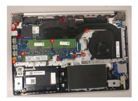
4 Release below cable: Speaker cable, DC-IN Cable, HDD cable, Finger Printer cable, backlight cable, TP cable , SD card cable, KB Cable, Power board cable ,EDP cable ,WWan antenna cable, Wlan antenna cable. And Disassemble Type-C BKT, RJ-45. Final step release main board
