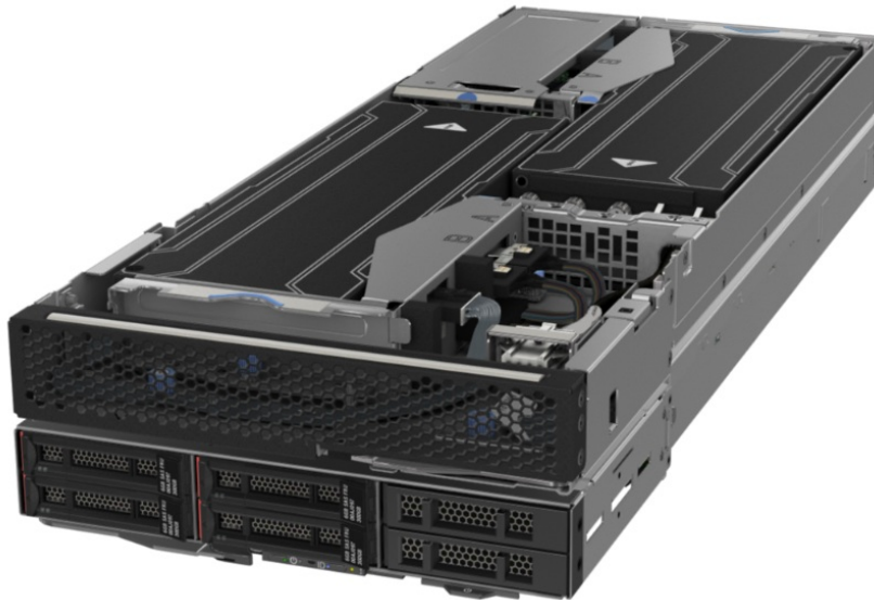
Figure 14. SD530 with GPU Tray attached
