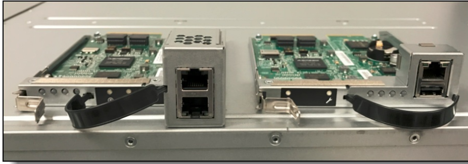
Figure 18. Dual-port SMM and standard (single-port) SMM
