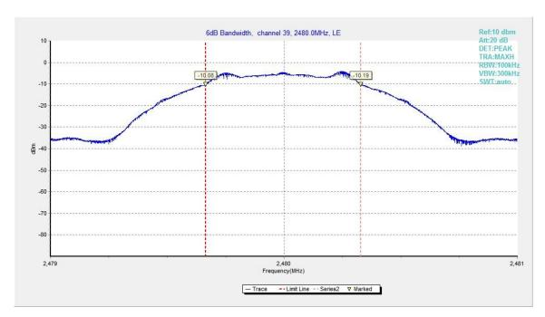
Fig.22. 6dB Bandwidth: GFSK, 2480 MHz
