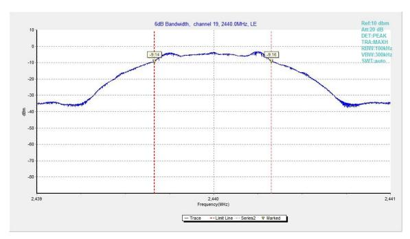
Fig.21. 6dB Bandwidth: GFSK, 2440 MHz
