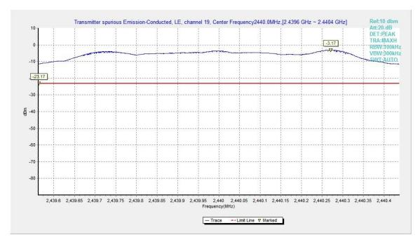
Fig.10. Transmitter Spurious Emission - Conducted: GFSK, 2440MHz
