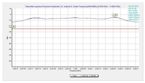
Fig.5. Transmitter Spurious Emission - Conducted: GFSK,2402MHz
