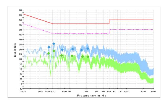
Fig.B.9.2 AC Powerline Conducted Emission-Idle
