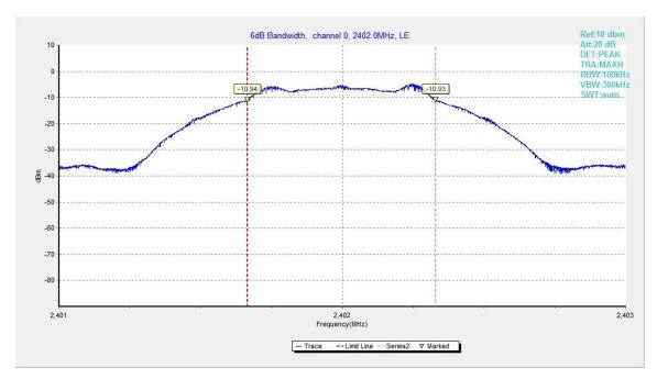
Fig.20. 6dB Bandwidth: GFSK, 2402 MHz
