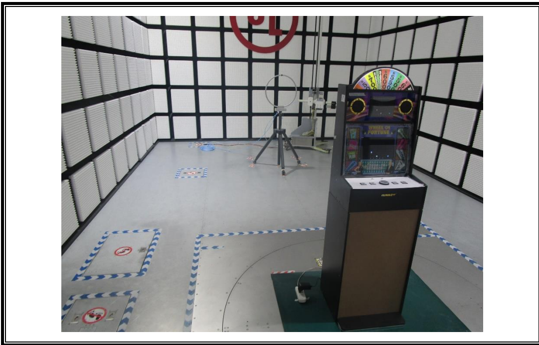
RADIATED RF MEASUREMENT SETUP (Below 30 MHz)
