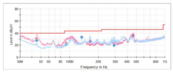
Frequency Quasi-Peak Limit Margin Height Azimuth Corr. Pol (MHz)  $(dB\mu V/m)$  $(dB\mu V/m)$ (dB) (cm) (deg) (dB/m)45.133100 27.56 40.00 12.44 100.0 V 98.0 -14.2 91.310200 20.55 43.50 22.95 100.0 V 98.0 -17.1 133.245850 32.79 43.50 10.71 200.0 Η 163.0 -11.7 162.438900 26.10 43.50 17.40 200.0 Н 18.0 -12.8 19.54 46.00 100.0 Н 341.0 292.088250 26.46 -10.7 462.911350 35.23 10.77 100.0 V 13.0 -7.1 46.00
