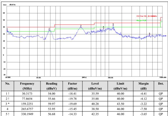
1). Emission level (dBuV/m) = 20 log Emission level (uV/m).
