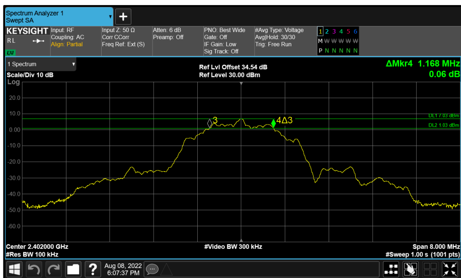
Figure 108 - BT Core 2 (C) 2402 MHz (CH37) 6 dB Bandwidth
