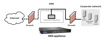
In both configurations, incoming requests to the SMA 6200/ 7200 services—including HTTP/S traffic for the Web proxy service—are sent over port 80 (HTTP) and port 443 (HTTPS). Traffic from the OnDemand agent is always sent over port 443. Because most networks are configured to enable traffic over these ports, you should not need to reconfigure firewalls on vour network.
