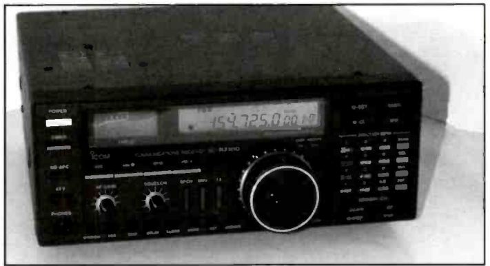
The ICOM R7100, with 1,000 memories, represents quite a leap forward. This receiver still shows up on the used market. Just be careful about which version you're buying.
