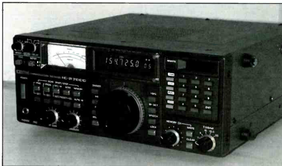
The ICOM R-7000 was the first high-end communications receiver widely available to hobbyists. Some swear by it as one of the most sensitive receivers ever built, while others swear it was one of the worst scanners.
