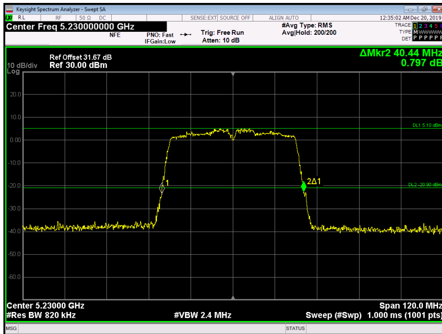
Figure 51 - 5230 MHz - 26 dB Emission Bandwidth
