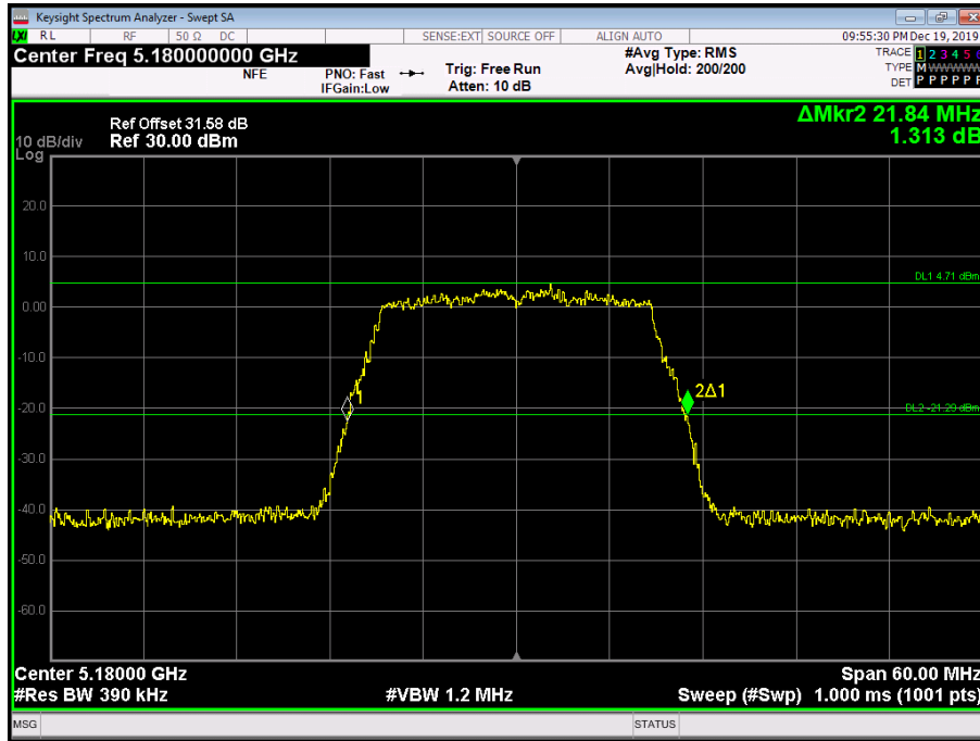
Figure 37 - 5180 MHz - 26 dB Emission Bandwidth
