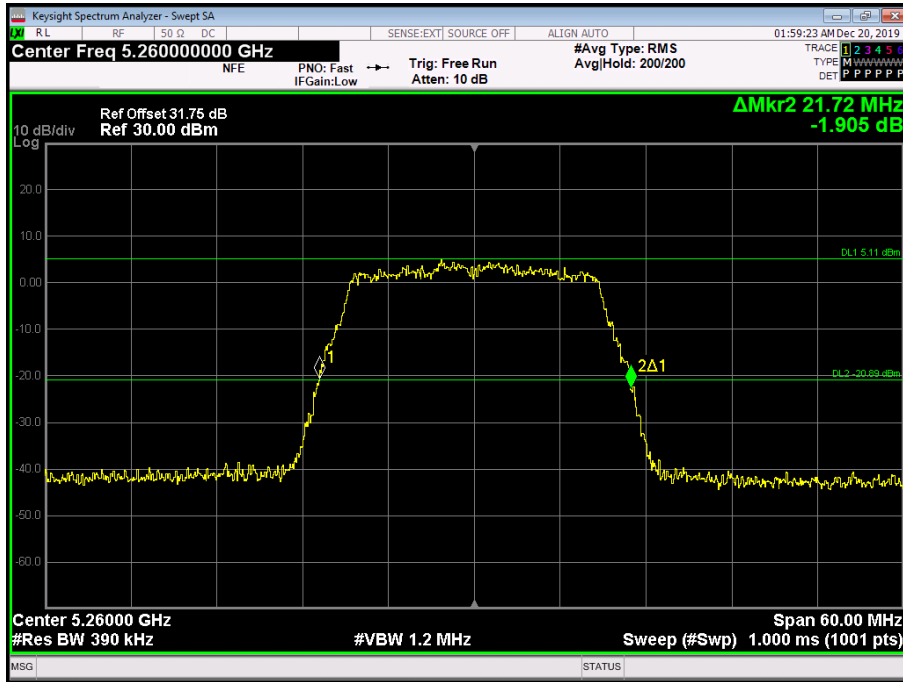
Figure 121 - 5260 MHz - 26 dB Emission Bandwidth
