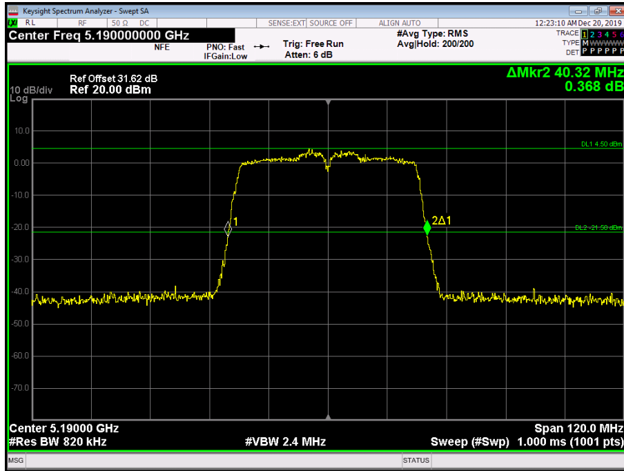
Figure 61 - 5190 MHz - 26 dB Emission Bandwidth
