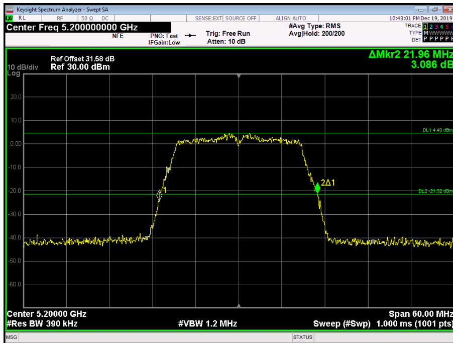
Figure 39 - 5200 MHz - 26 dB Emission Bandwidth
