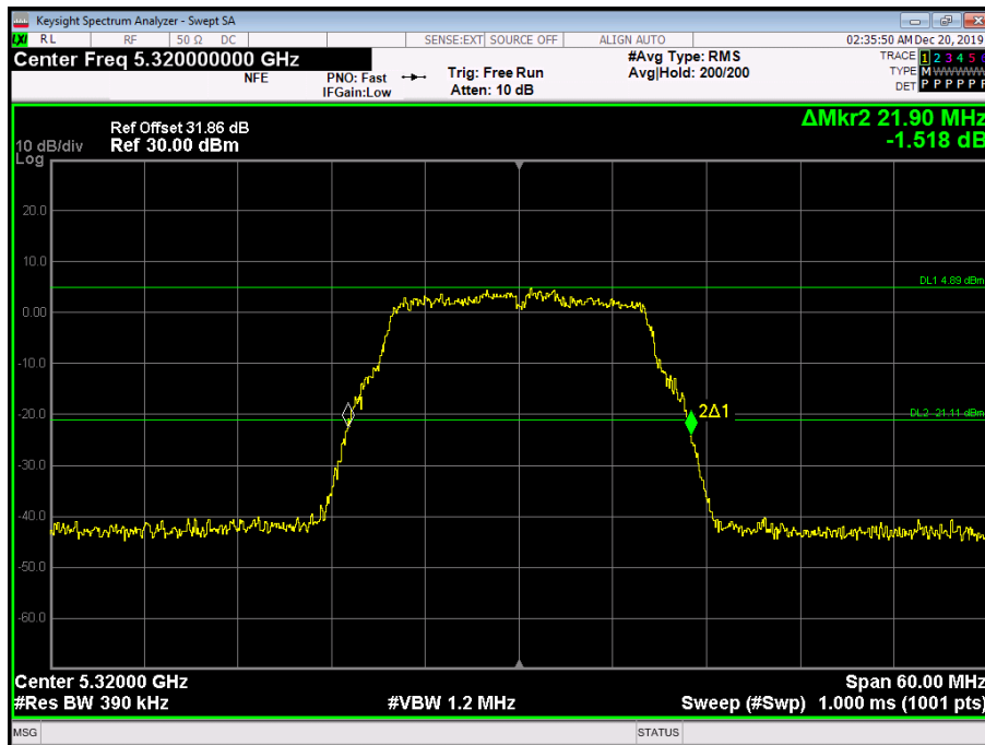
Figure 113 - 5320 MHz - 26 dB Emission Bandwidth
