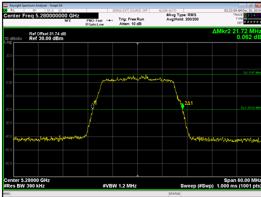
Figure 123 - 5280 MHz - 26 dB Emission Bandwidth
