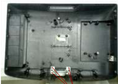
1.13The ninth of TV teardown --Tearing down the Base Axis
