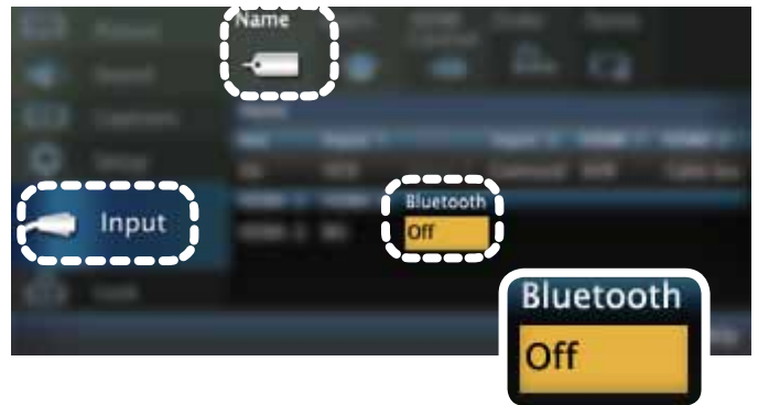
Remove the Bluetooth icon from the Input Selection menu by turning off Bluetooth in the Input > Name menu.
