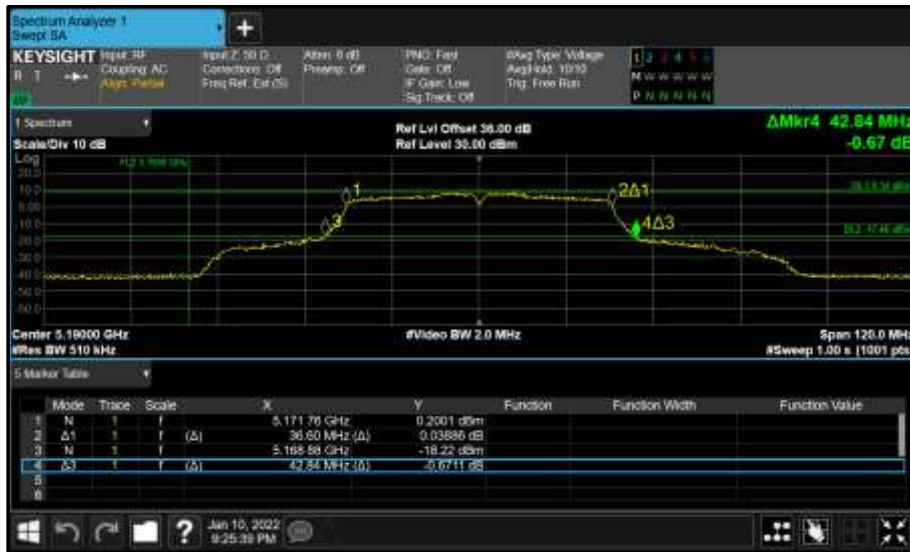
Figure 129 - Core 0 (A) 5190 MHz (CH38) 26 dB and 99% Bandwidth
