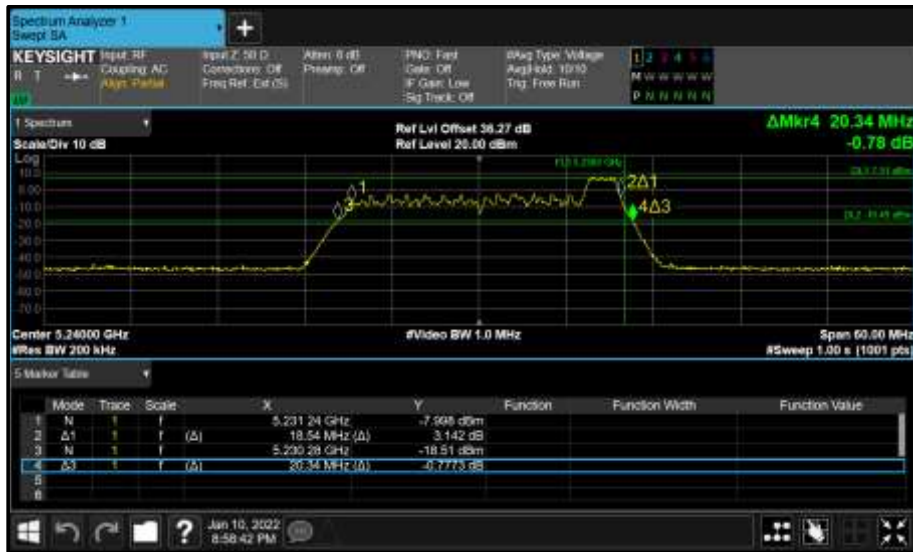
Figure 186 - Core 0 (A) 5240 MHz (CH48) 26 dB and 99% Bandwidth
