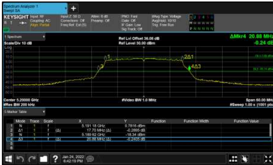
Figure 111 - Core 0 (A) 5200 MHz (CH40) 26 dB and 99% Bandwidth
