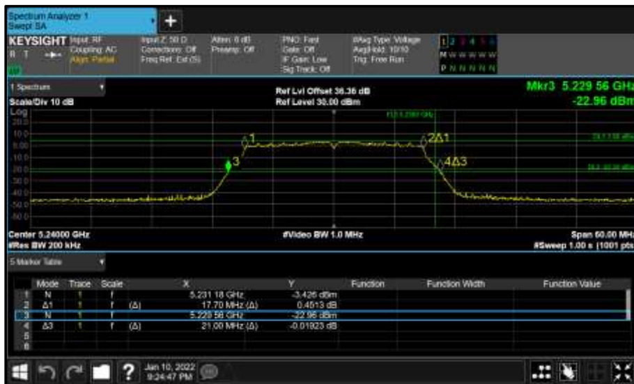
Figure 108 - Core 1 (B) 5240 MHz (CH48) 26 dB and 99% Bandwidth
