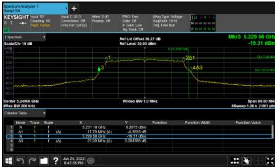
Figure 113 - Core 0 (A) 5240 MHz (CH48) 26 dB and 99% Bandwidth
