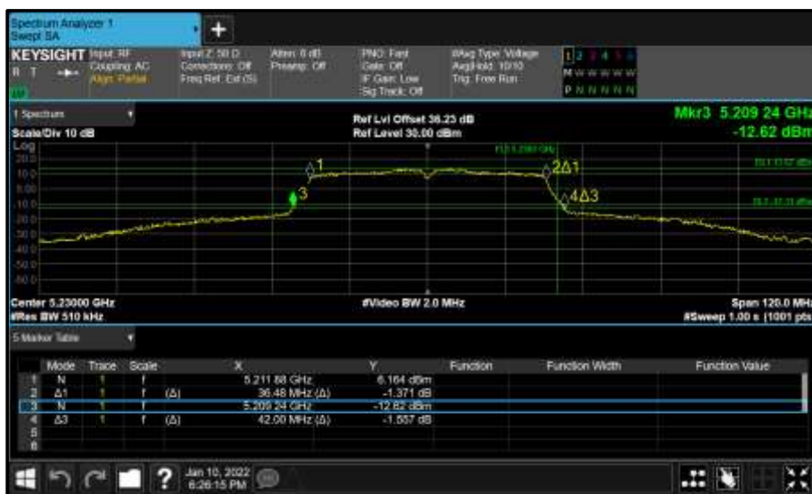
Figure 122 - Core 0 (A) 5230 MHz (CH46) 26 dB and 99% Bandwidth
