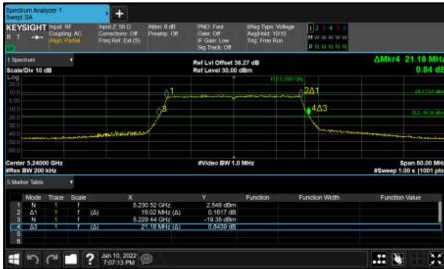
Figure 161 - Core 0 (A) 5240 MHz (CH48) 26 dB and 99% Bandwidth
