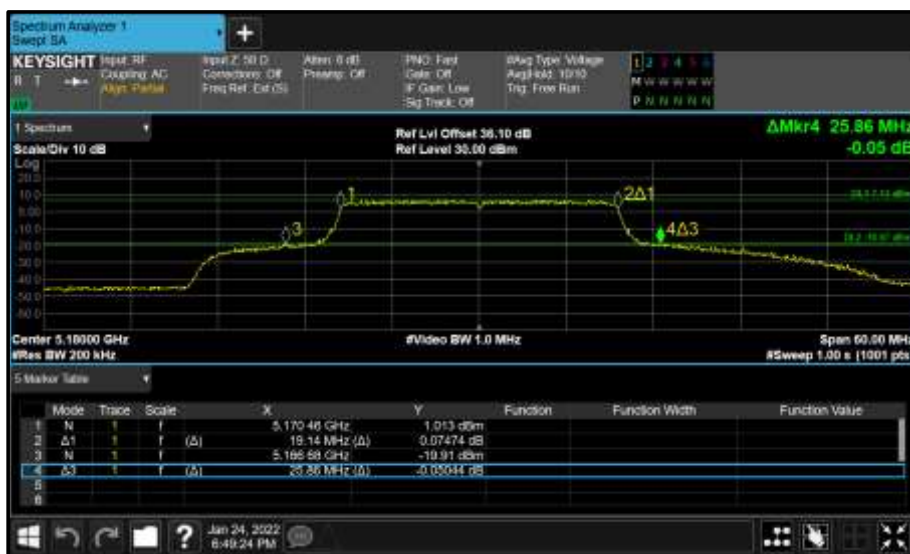
Figure 170 - Core 1 (B) 5180 MHz (CH36) 26 dB and 99% Bandwidth
