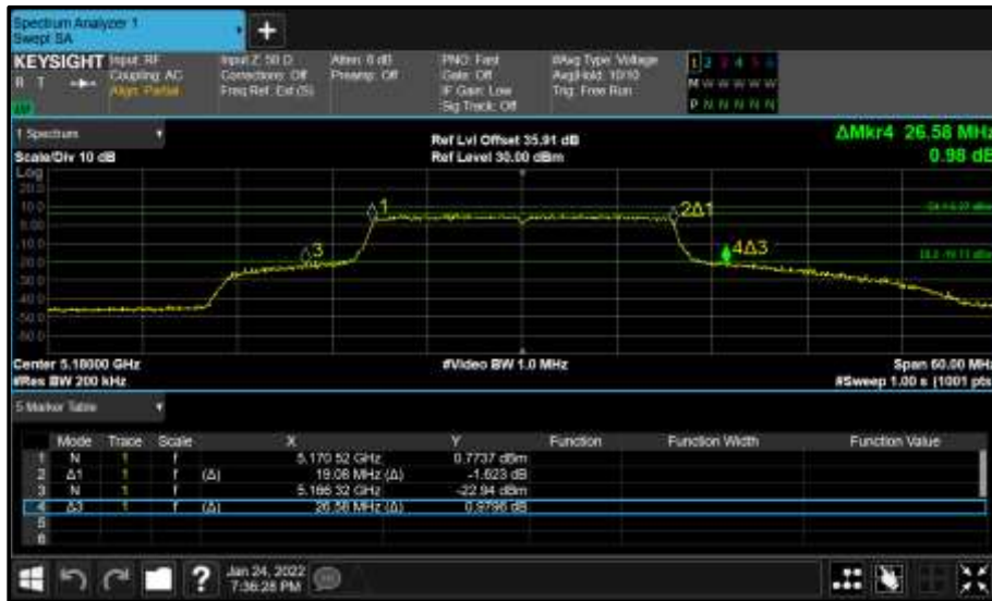
Figure 175 - Core 0 (A) 5180 MHz (CH36) 26 dB and 99% Bandwidth
