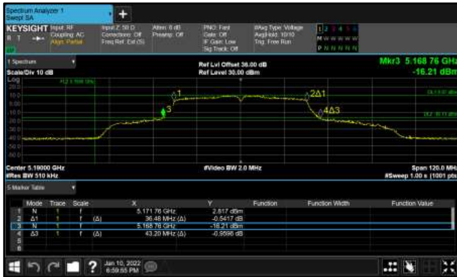
Figure 125 - Core 0 (A) 5190 MHz (CH38) 26 dB and 99% Bandwidth
