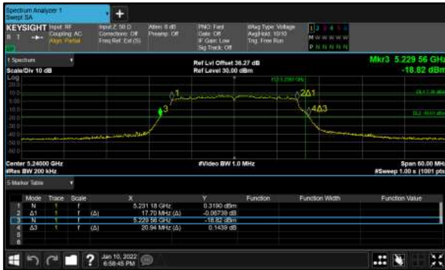
Figure 101 - Core 0 (A) 5240 MHz (CH48) 26 dB and 99% Bandwidth
