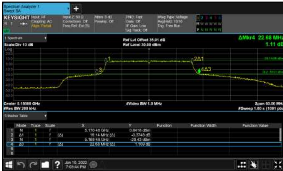
Figure 157 - Core 0 (A) 5180 MHz (CH36) 26 dB and 99% Bandwidth
