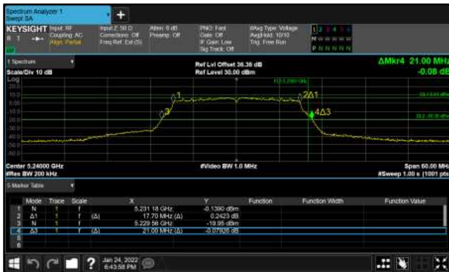
Figure 114 - Core 1 (B) 5240 MHz (CH48) 26 dB and 99% Bandwidth
