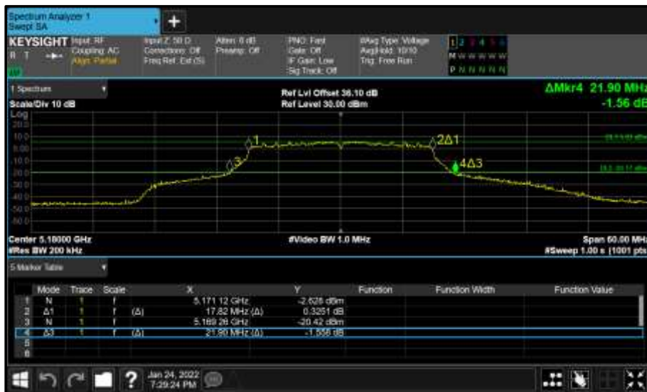
Figure 116 - Core 1 (B) 5180 MHz (CH36) 26 dB and 99% Bandwidth
