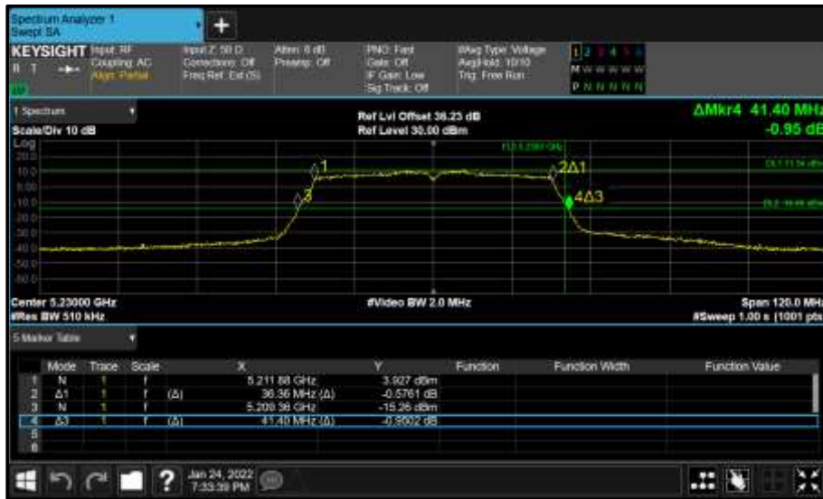
Figure 139 - Core 0 (A) 5230 MHz (CH46) 26 dB and 99% Bandwidth
