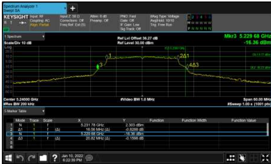
Figure 87 - Core 0 (A) 5240 MHz (CH48) 26 dB and 99% Bandwidth
