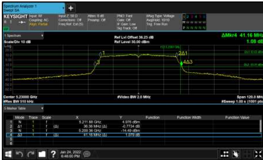
Figure 135 - Core 0 (A) 5230 MHz (CH46) 26 dB and 99% Bandwidth
