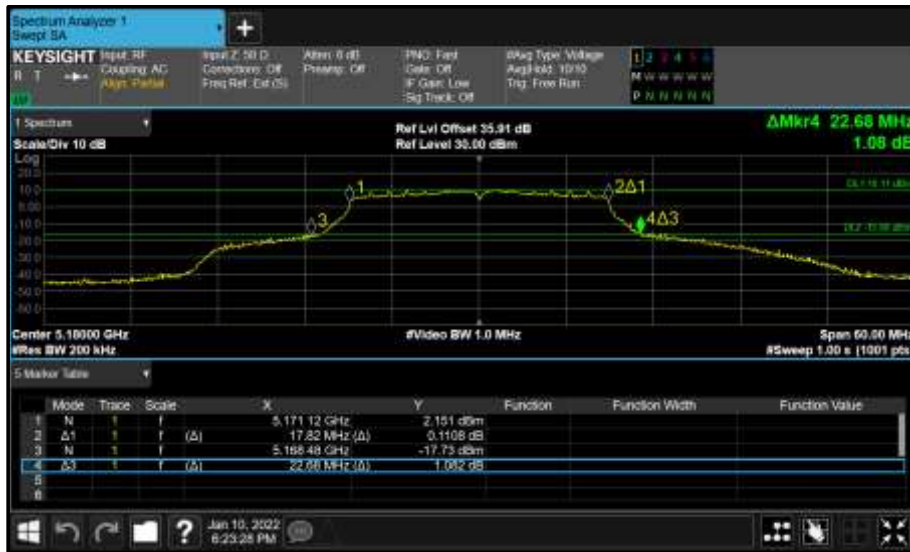
Figure 91 - Core 0 (A) 5180 MHz (CH36) 26 dB and 99% Bandwidth
