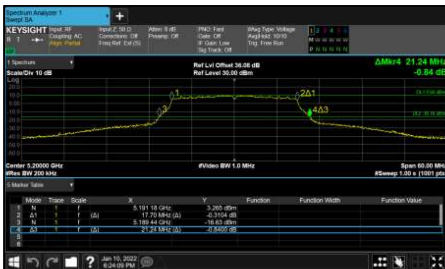
Figure 92 - Core 0 (A) 5200 MHz (CH40) 26 dB and 99% Bandwidth
