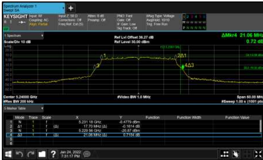
Figure 119 - Core 0 (A) 5240 MHz (CH48) 26 dB and 99% Bandwidth
