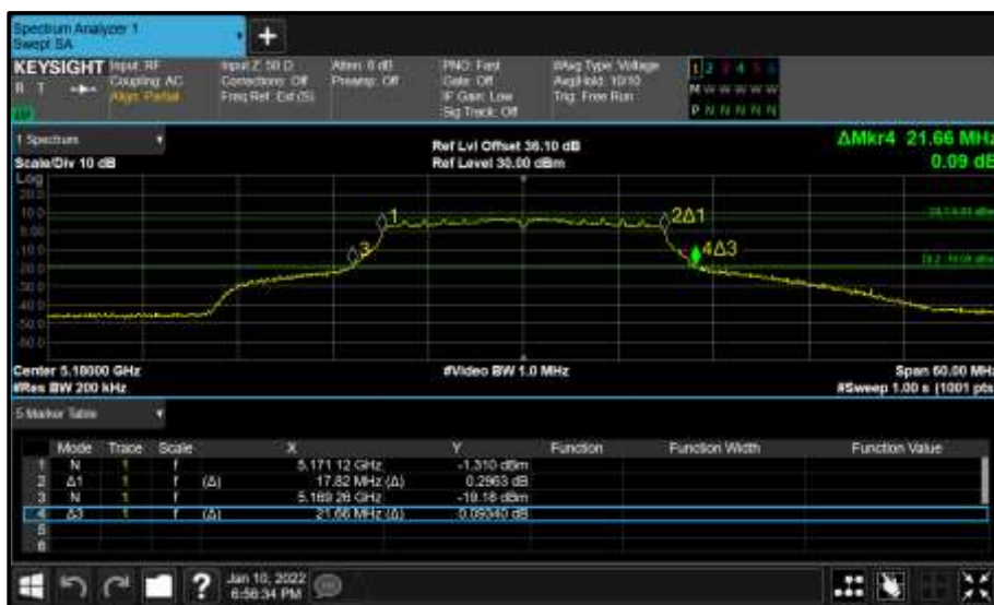
Figure 98 - Core 1 (B) 5180 MHz (CH36) 26 dB and 99% Bandwidth
