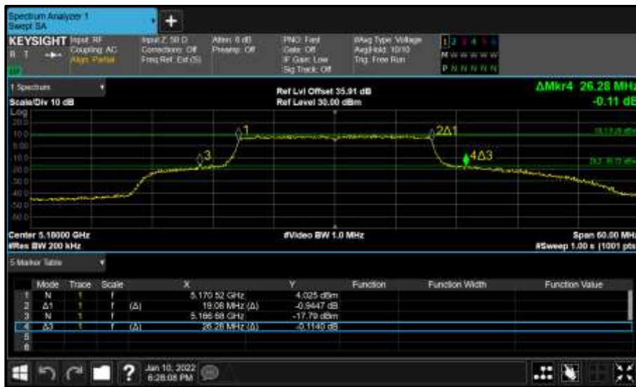
Figure 151 - Core 0 (A) 5180 MHz (CH36) 26 dB and 99% Bandwidth
