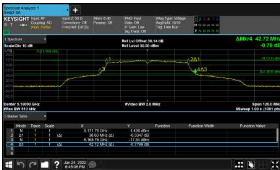
Figure 134 - Core 1 (B) 5190 MHz (CH38) 26 dB and 99% Bandwidth
