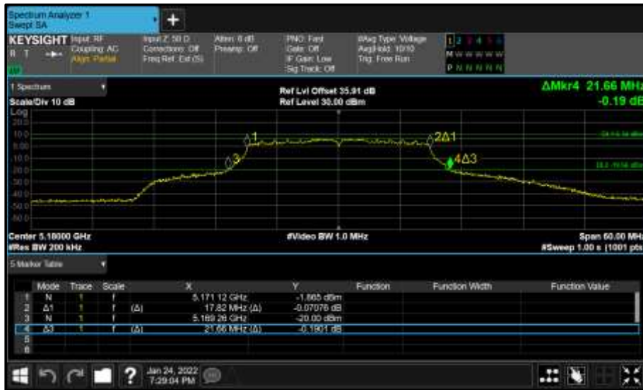
Figure 115 - Core 0 (A) 5180 MHz (CH36) 26 dB and 99% Bandwidth
