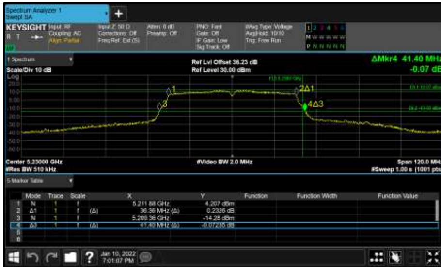
Figure 127 - Core 0 (A) 5230 MHz (CH46) 26 dB and 99% Bandwidth
