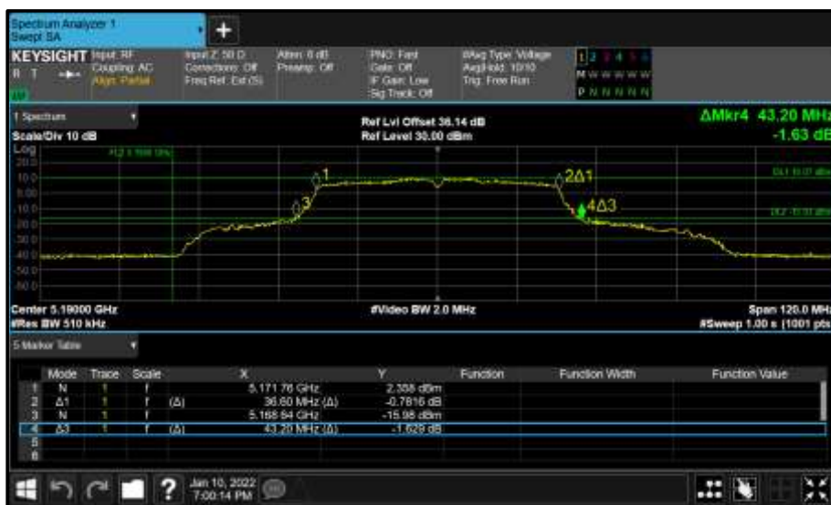
Figure 126 - Core 1 (B) 5190 MHz (CH38) 26 dB and 99% Bandwidth
