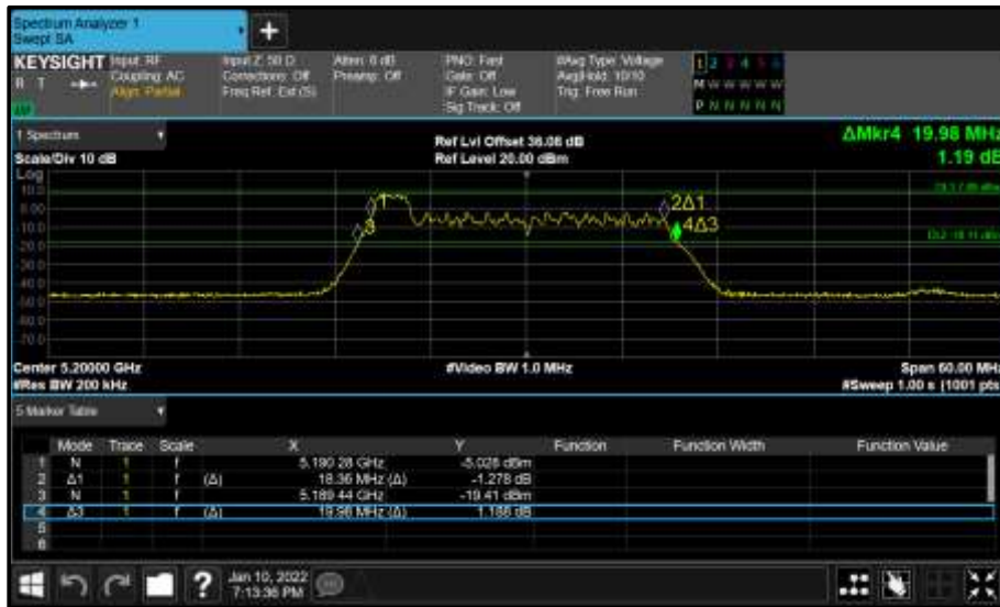
Figure 189 - Core 0 (A) 5200 MHz (CH40) 26 dB and 99% Bandwidth
