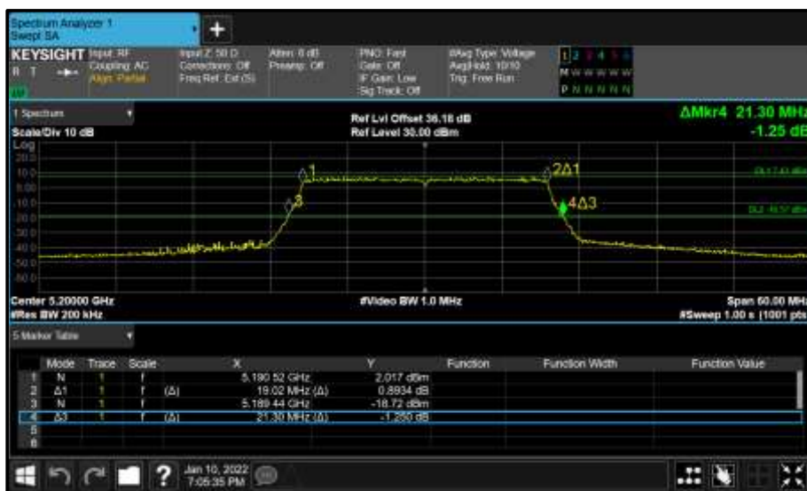
Figure 160 - Core 1 (B) 5200 MHz (CH40) 26 dB and 99% Bandwidth
