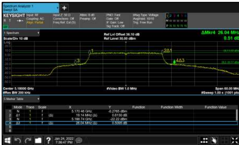
Figure 176 - Core 1 (B) 5180 MHz (CH36) 26 dB and 99% Bandwidth
