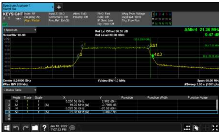
Figure 162 - Core 1 (B) 5240 MHz (CH48) 26 dB and 99% Bandwidth
