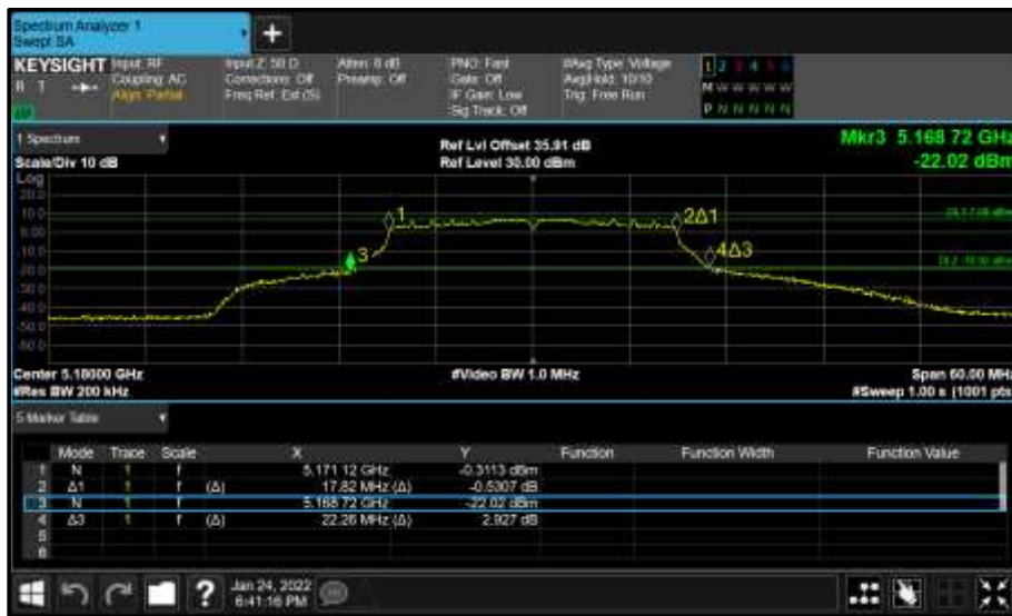
Figure 109 - Core 0 (A) 5180 MHz (CH36) 26 dB and 99% Bandwidth
