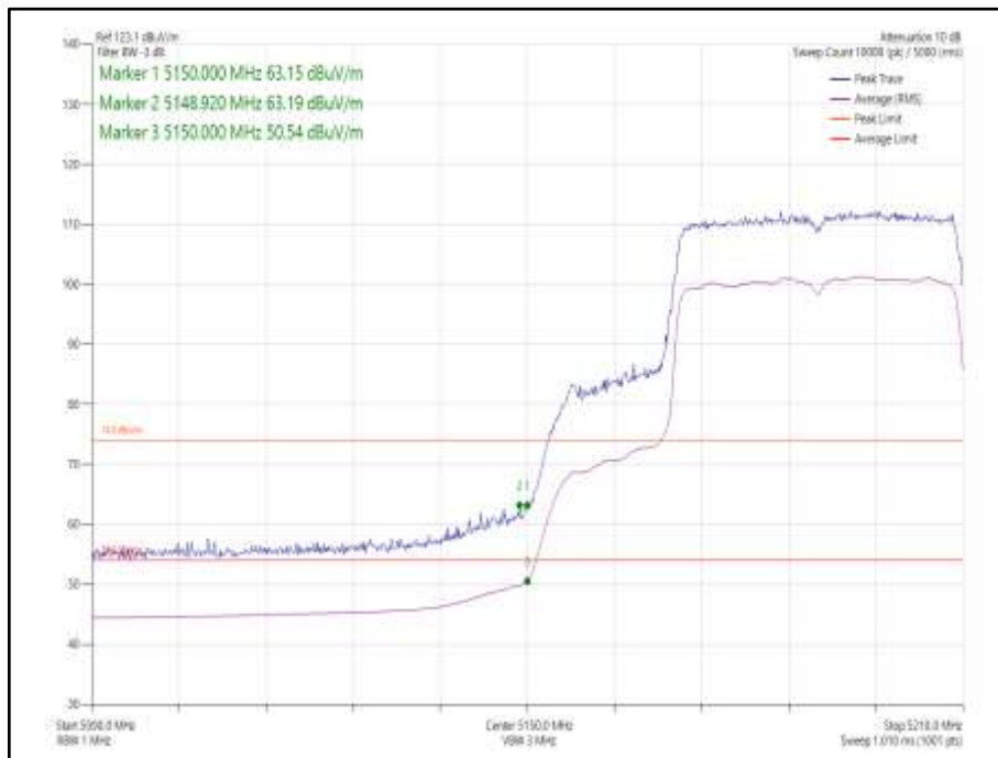
Figure 44 802.11ax HE40 SDM, Cores 0-1, SU - 5190 MHz Band Edge Frequency 5150 MHz
