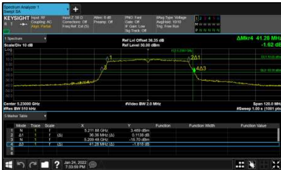
Figure 140 - Core 1 (B) 5230 MHz (CH46) 26 dB and 99% Bandwidth
