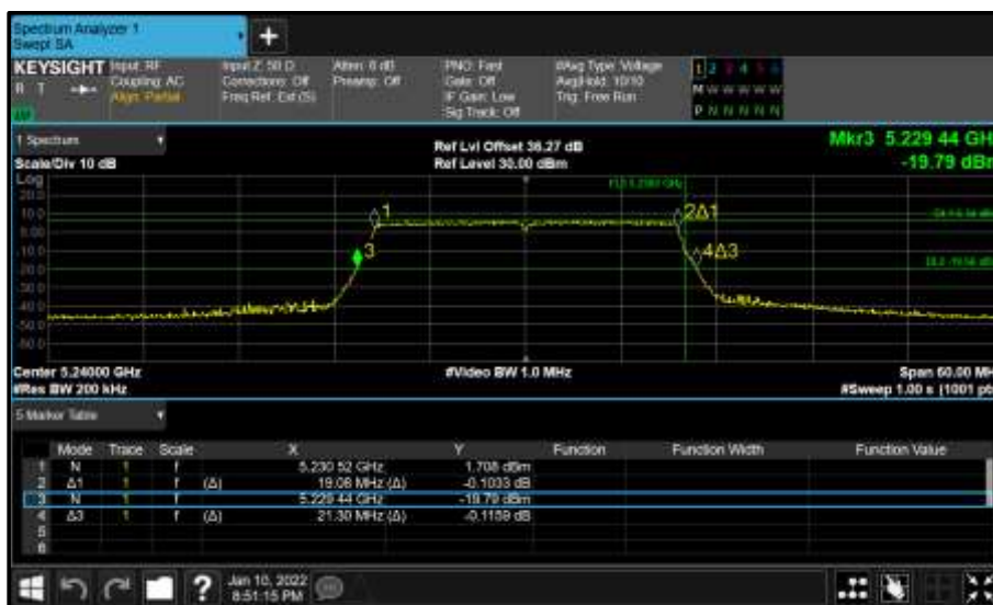
Figure 156 - Core 0 (A) 5240 MHz (CH48) 26 dB and 99% Bandwidth
