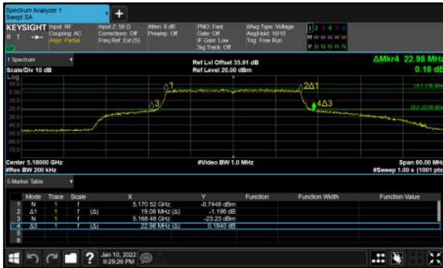
Figure 163 - Core 0 (A) 5180 MHz (CH36) 26 dB and 99% Bandwidth
