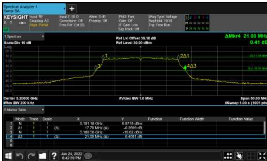
Figure 112 - Core 1 (B) 5200 MHz (CH40) 26 dB and 99% Bandwidth
