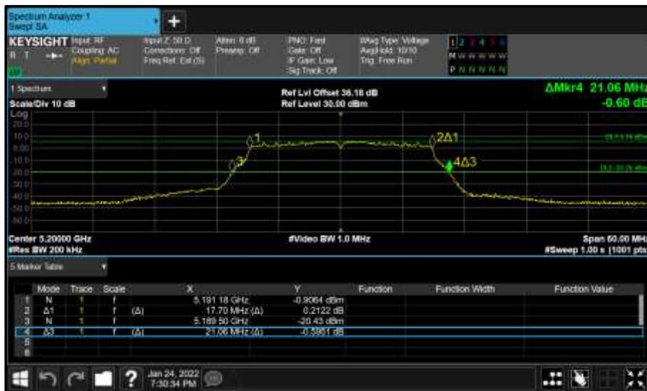
Figure 118 - Core 1 (B) 5200 MHz (CH40) 26 dB and 99% Bandwidth
