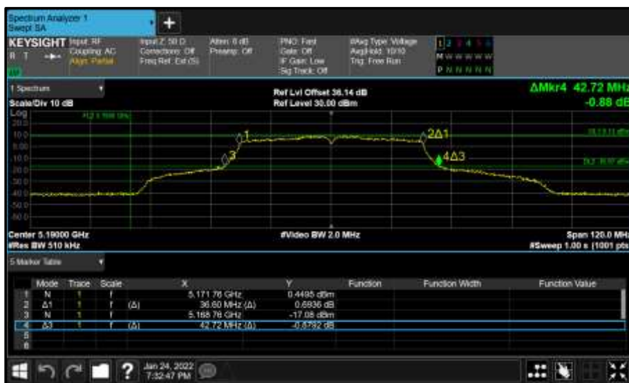
Figure 138 - Core 1 (B) 5190 MHz (CH38) 26 dB and 99% Bandwidth
