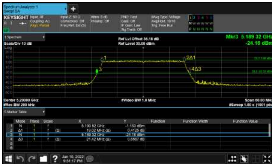
Figure 166 - Core 1 (B) 5200 MHz (CH40) 26 dB and 99% Bandwidth
