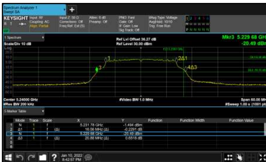
Figure 90 - Core 0 (A) 5240 MHz (CH48) 26 dB and 99% Bandwidth
