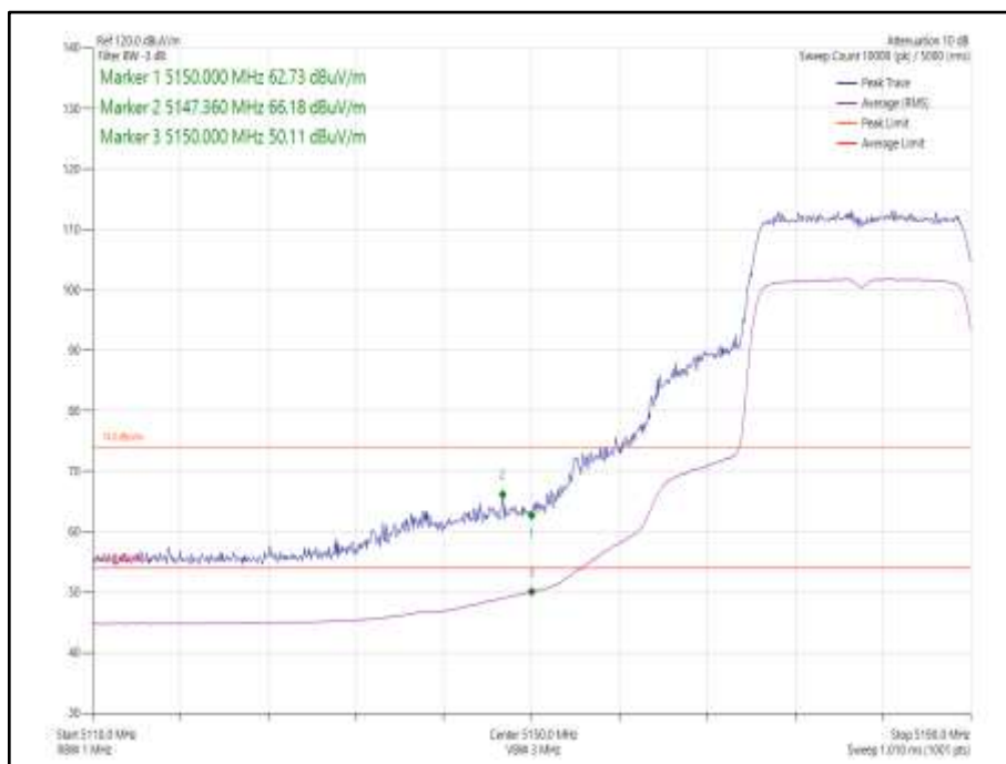
Figure 3 - 802.11ax HE20, Core 1, SU - 5180 MHz, Band Edge Frequency 5150 MHz
