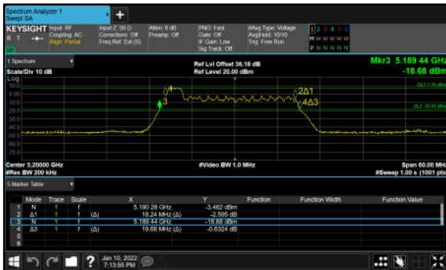
Figure 190 - Core 1 (B) 5200 MHz (CH40) 26 dB and 99% Bandwidth
