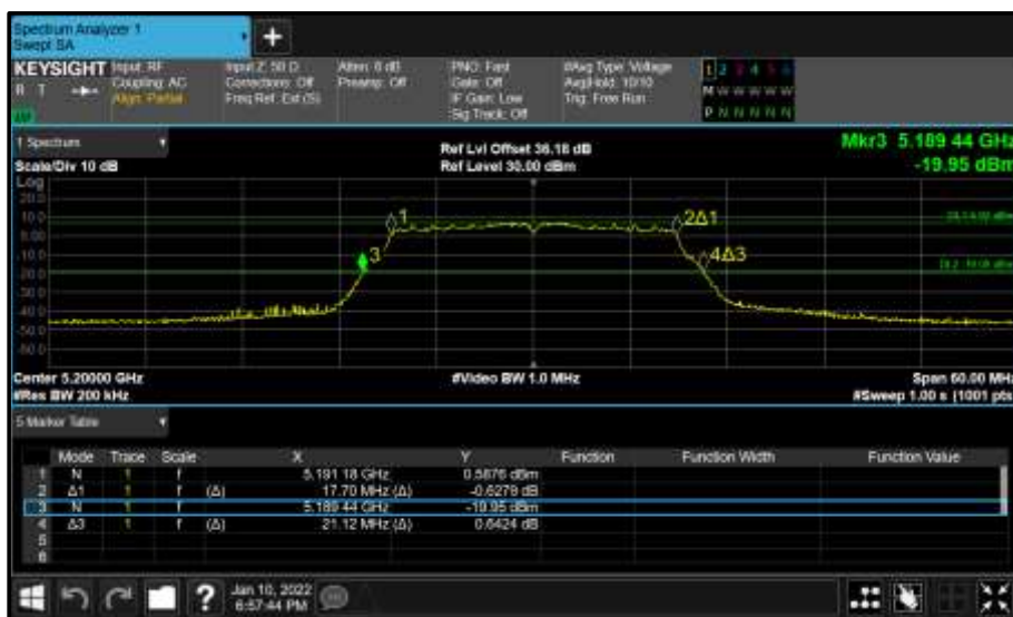
Figure 100 - Core 1 (B) 5200 MHz (CH40) 26 dB and 99% Bandwidth
