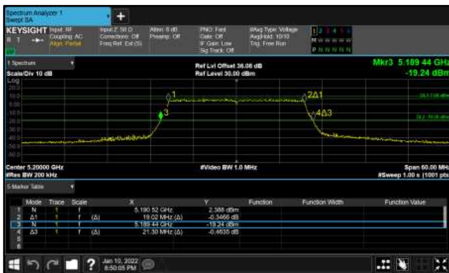
Figure 155 - Core 0 (A) 5200 MHz (CH40) 26 dB and 99% Bandwidth
