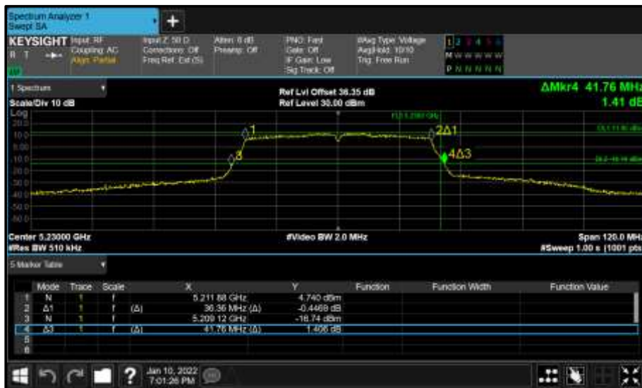
Figure 128 - Core 1 (B) 5230 MHz (CH46) 26 dB and 99% Bandwidth
