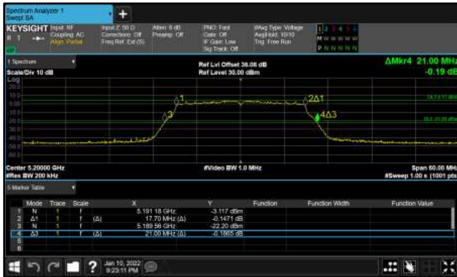
Figure 105 - Core 0 (A) 5200 MHz (CH40) 26 dB and 99% Bandwidth
