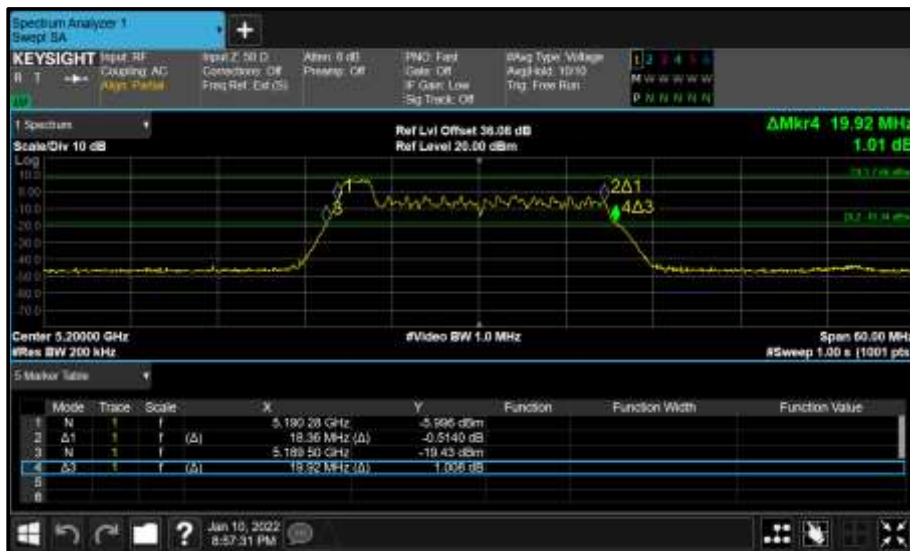
Figure 185 - Core 0 (A) 5200 MHz (CH40) 26 dB and 99% Bandwidth
