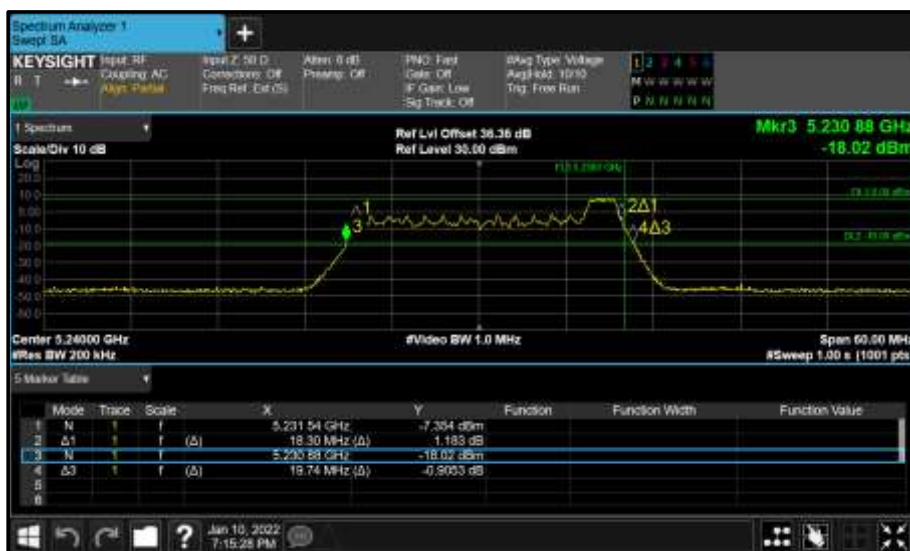
Figure 192 - Core 1 (B) 5240 MHz (CH48) 26 dB and 99% Bandwidth
