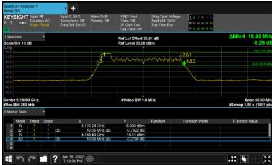
Figure 187 - Core 0 (A) 5180 MHz (CH36) 26 dB and 99% Bandwidth
