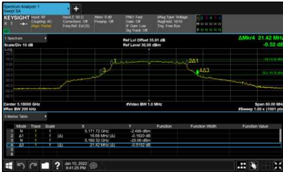
Figure 88 - Core 0 (A) 5180 MHz (CH36) 26 dB and 99% Bandwidth
