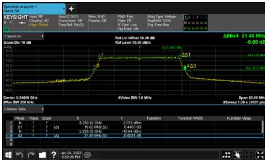
Figure 174 - Core 1 (B) 5240 MHz (CH48) 26 dB and 99% Bandwidth
