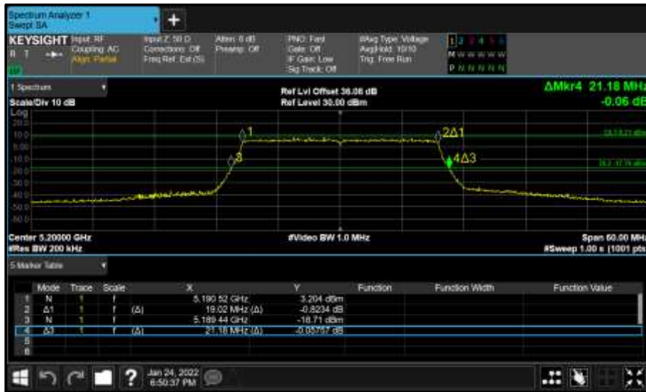
Figure 171 - Core 0 (A) 5200 MHz (CH40) 26 dB and 99% Bandwidth
