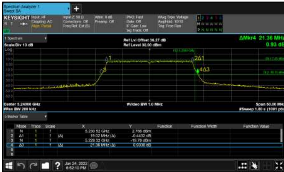
Figure 173 - Core 0 (A) 5240 MHz (CH48) 26 dB and 99% Bandwidth
