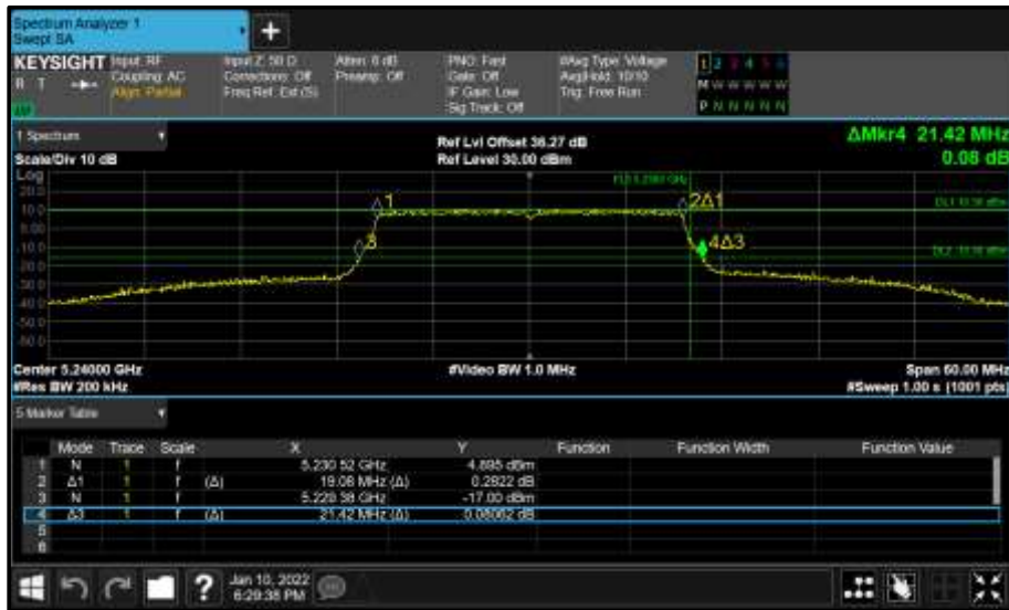
Figure 153 - Core 0 (A) 5240 MHz (CH48) 26 dB and 99% Bandwidth
