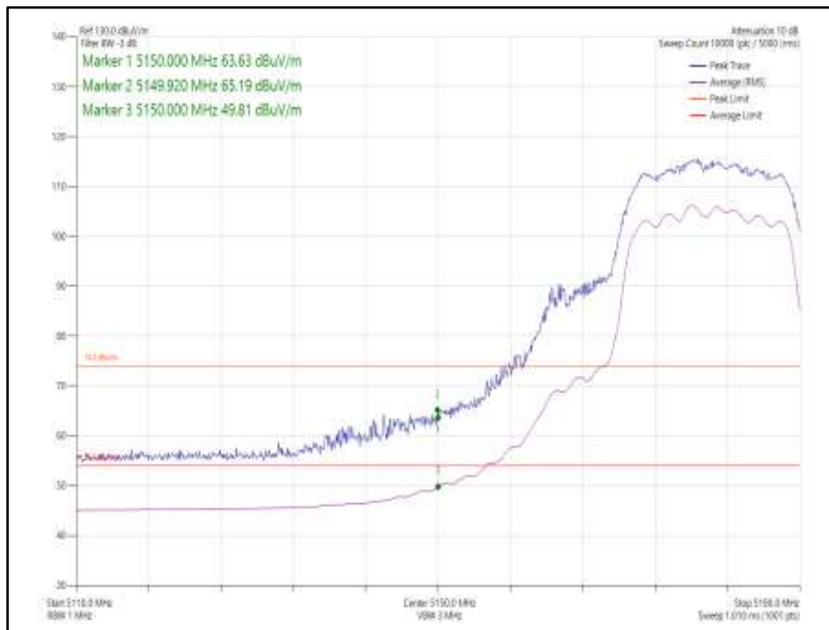
Figure 13 - 802.11n HT20 CDD, Cores 0-1 - 5180 MHz Band Edge Frequency 5150 MHz
