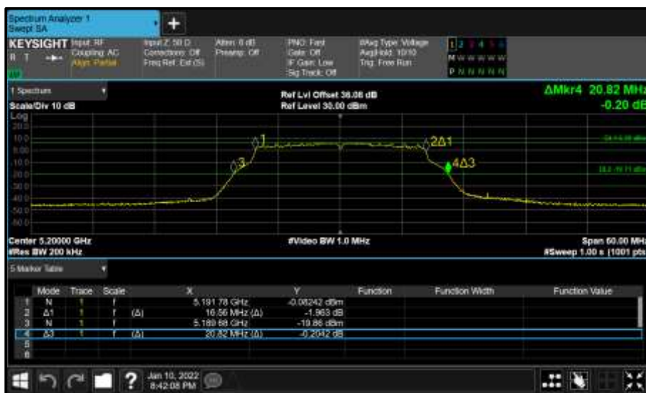
Figure 89 - Core 0 (A) 5200 MHz (CH40) 26 dB and 99% Bandwidth
