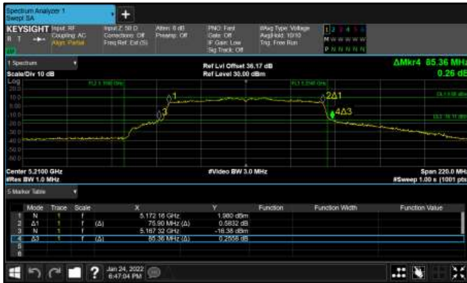
Figure 147 - Core 0 (A) 5210 MHz (CH42) 26 dB and 99% Bandwidth
