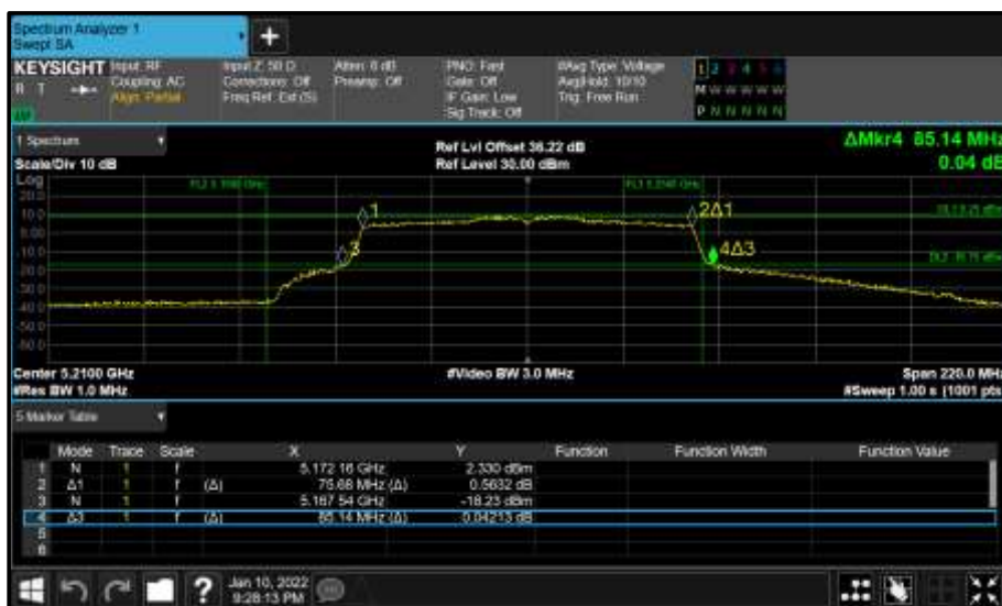
Figure 146 - Core 1 (B) 5210 MHz (CH42) 26 dB and 99% Bandwidth
