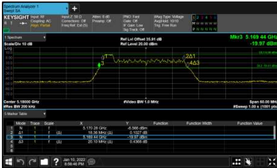
Figure 184 - Core 0 (A) 5180 MHz (CH36) 26 dB and 99% Bandwidth
