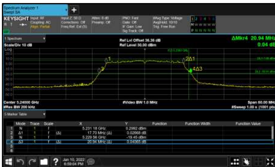
Figure 102 - Core 1 (B) 5240 MHz (CH48) 26 dB and 99% Bandwidth
