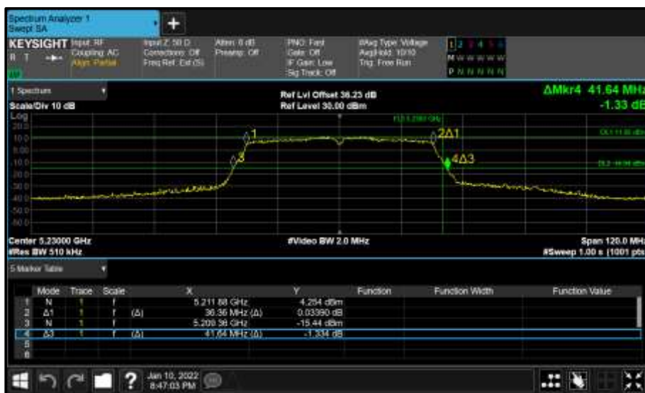
Figure 124 - Core 0 (A) 5230 MHz (CH46) 26 dB and 99% Bandwidth
