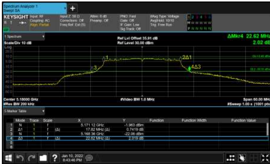
Figure 94 - Core 0 (A) 5180 MHz (CH36) 26 dB and 99% Bandwidth
