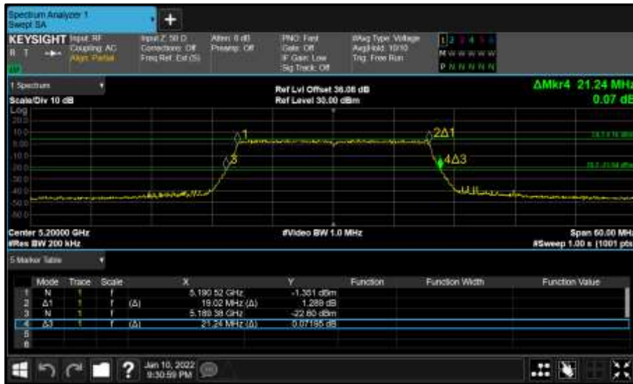
Figure 165 - Core 0 (A) 5200 MHz (CH40) 26 dB and 99% Bandwidth
