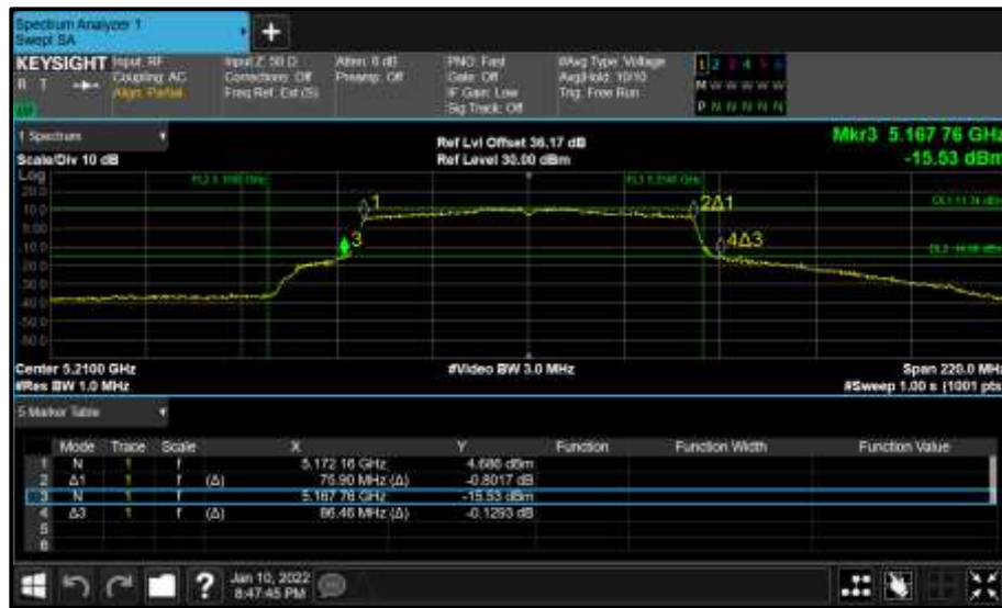
Figure 142 - Core 0 (A) 5210 MHz (CH42) 26 dB and 99% Bandwidth
