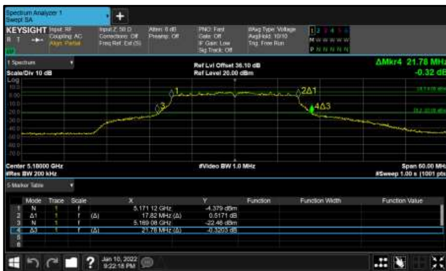
Figure 104 - Core 1 (B) 5180 MHz (CH36) 26 dB and 99% Bandwidth
