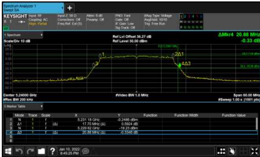
Figure 96 - Core 0 (A) 5240 MHz (CH48) 26 dB and 99% Bandwidth
