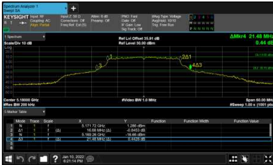
Figure 85 - Core 0 (A) 5180 MHz (CH36) 26 dB and 99% Bandwidth
