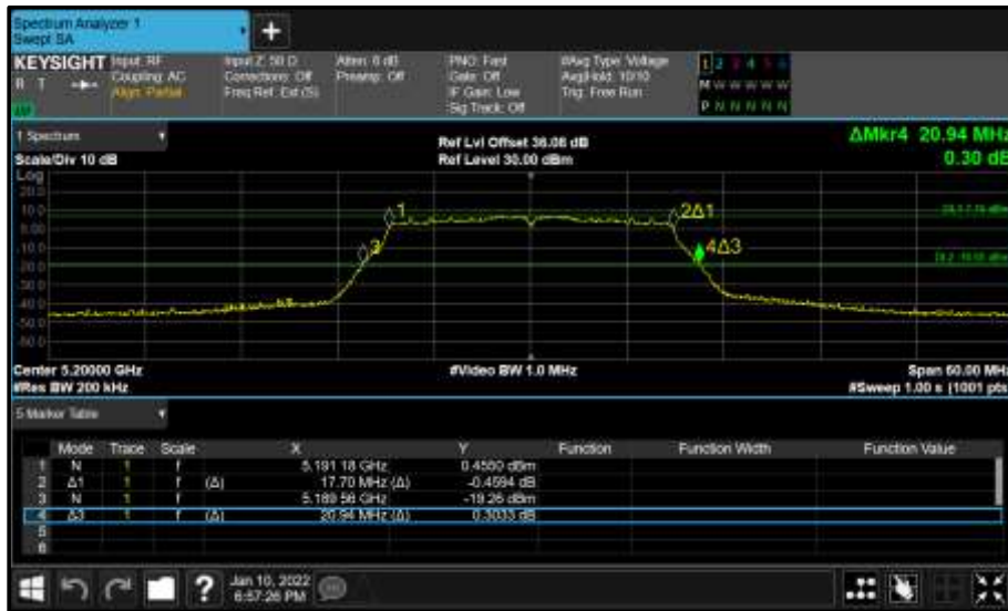
Figure 99 - Core 0 (A) 5200 MHz (CH40) 26 dB and 99% Bandwidth
