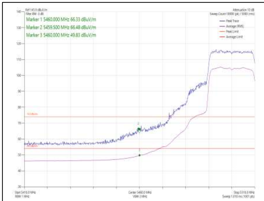
Figure 29 - 802.11ax HE20 SDM, Cores 0-1, SU- 5500 MHz Band Edge Frequency 5460 MHz
