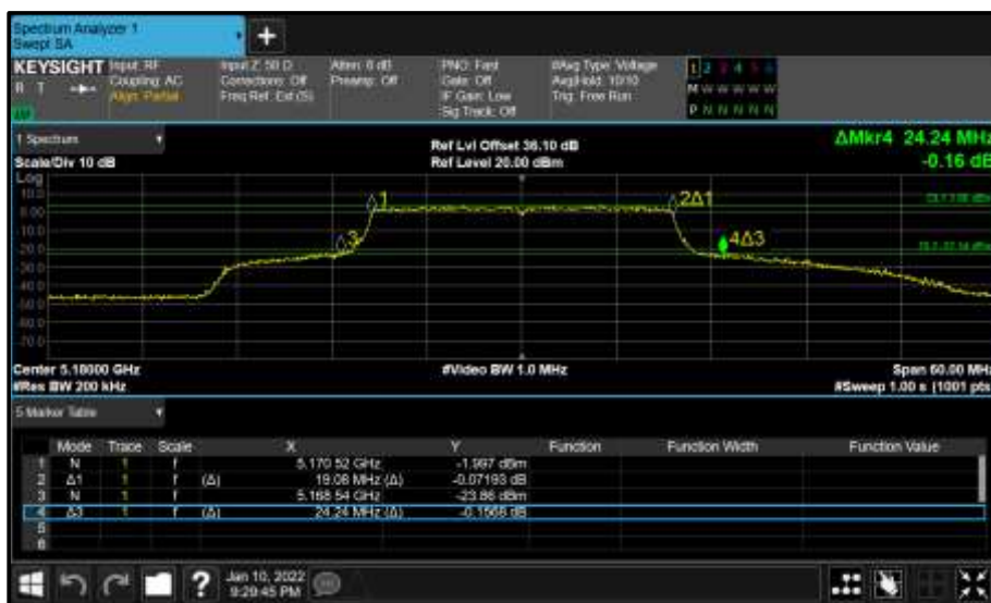
Figure 164 - Core 1 (B) 5180 MHz (CH36) 26 dB and 99% Bandwidth
