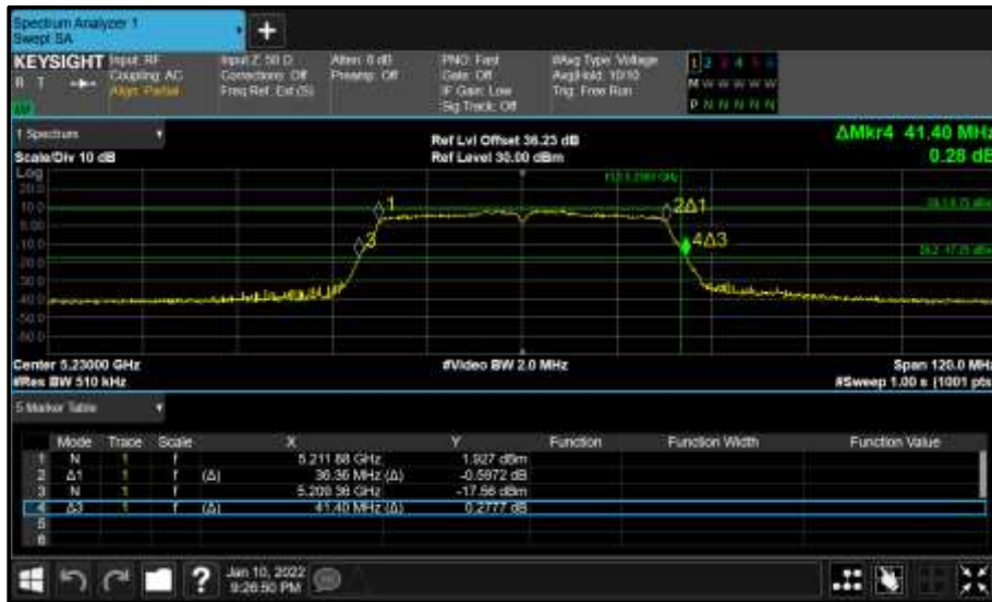
Figure 131 - Core 0 (A) 5230 MHz (CH46) 26 dB and 99% Bandwidth
