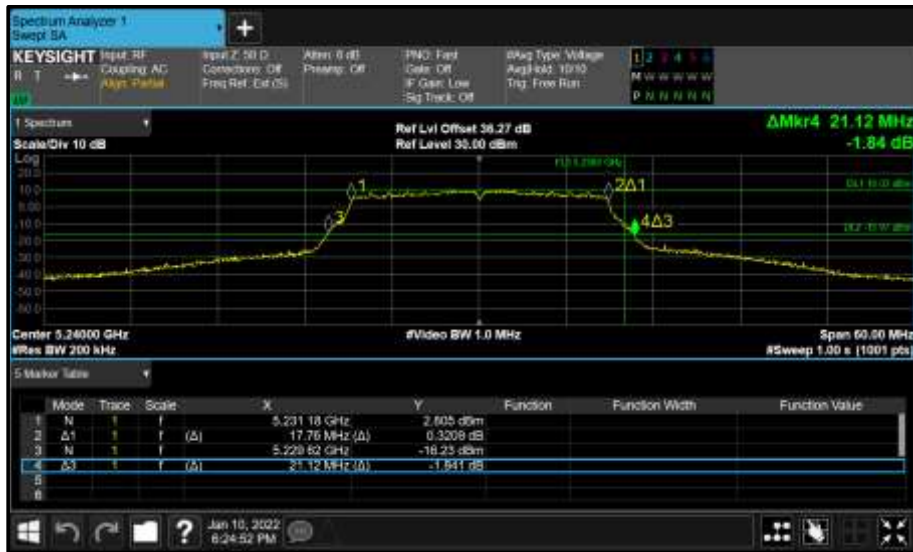
Figure 93 - Core 0 (A) 5240 MHz (CH48) 26 dB and 99% Bandwidth
