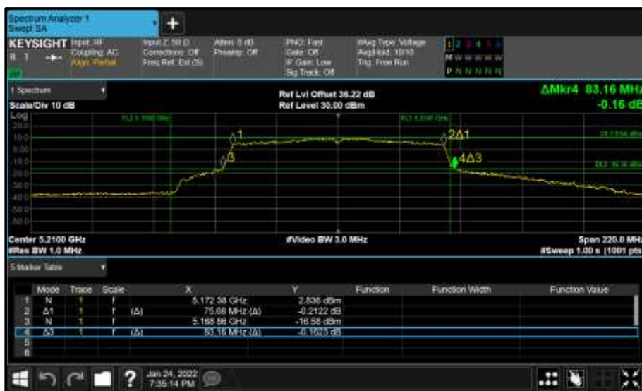
Figure 150 - Core 1 (B) 5210 MHz (CH42) 26 dB and 99% Bandwidth
