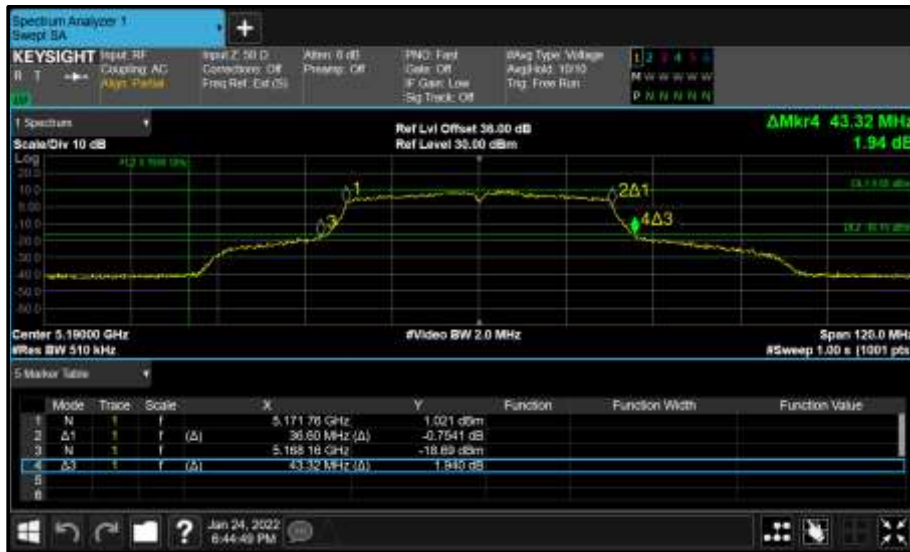
Figure 133 - Core 0 (A) 5190 MHz (CH38) 26 dB and 99% Bandwidth
