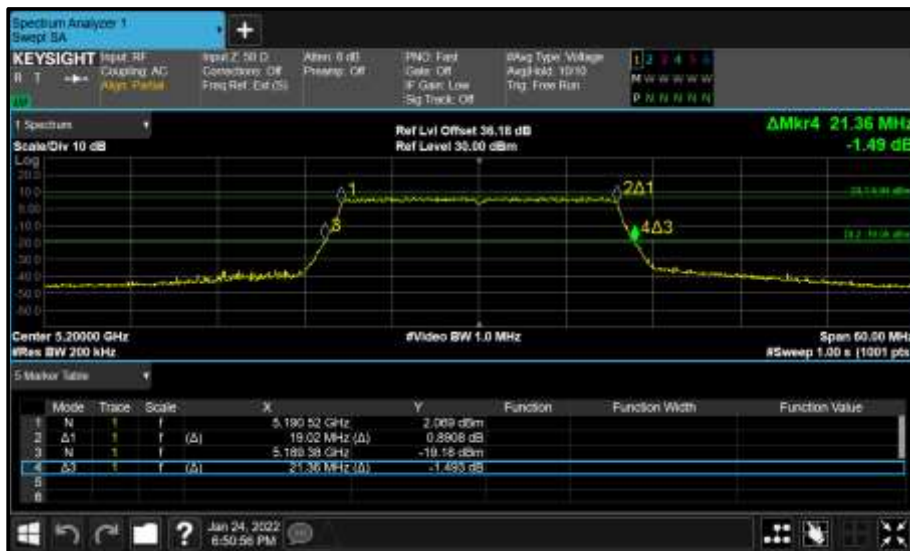
Figure 172 - Core 1 (B) 5200 MHz (CH40) 26 dB and 99% Bandwidth
