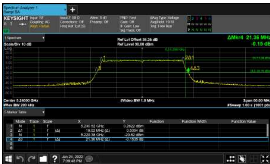
Figure 180 - Core 1 (B) 5240 MHz (CH48) 26 dB and 99% Bandwidth
