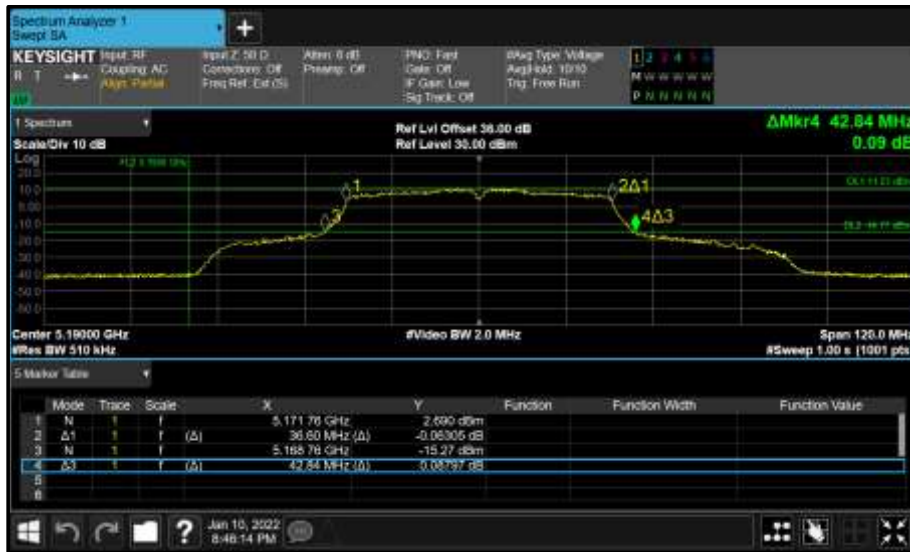
Figure 123 - Core 0 (A) 5190 MHz (CH38) 26 dB and 99% Bandwidth
