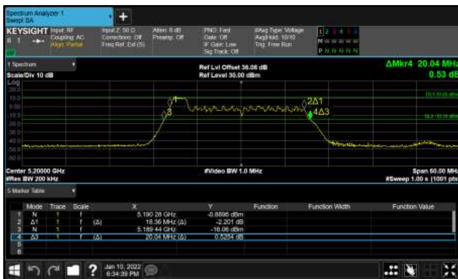
Figure 182 - Core 0 (A) 5200 MHz (CH40) 26 dB and 99% Bandwidth
