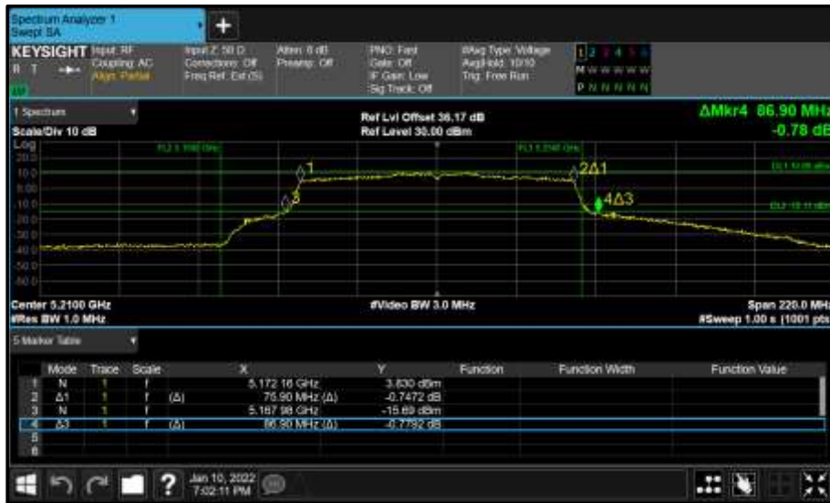
Figure 143 - Core 0 (A) 5210 MHz (CH42) 26 dB and 99% Bandwidth
