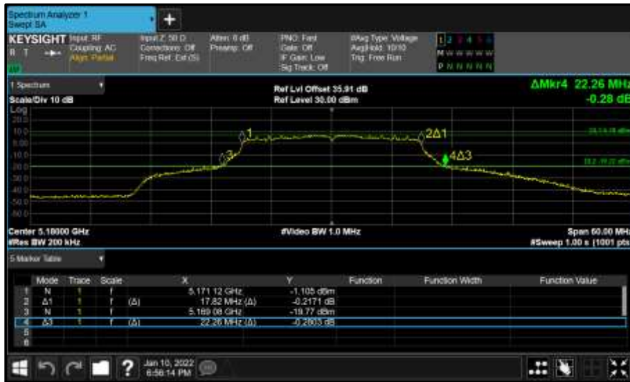
Figure 97 - Core 0 (A) 5180 MHz (CH36) 26 dB and 99% Bandwidth
