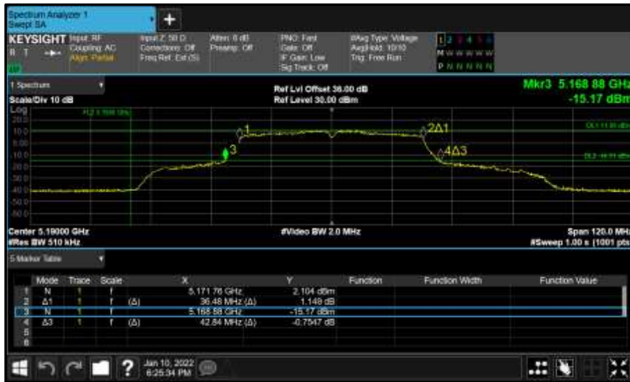
Figure 121 - Core 0 (A) 5190 MHz (CH38) 26 dB and 99% Bandwidth
