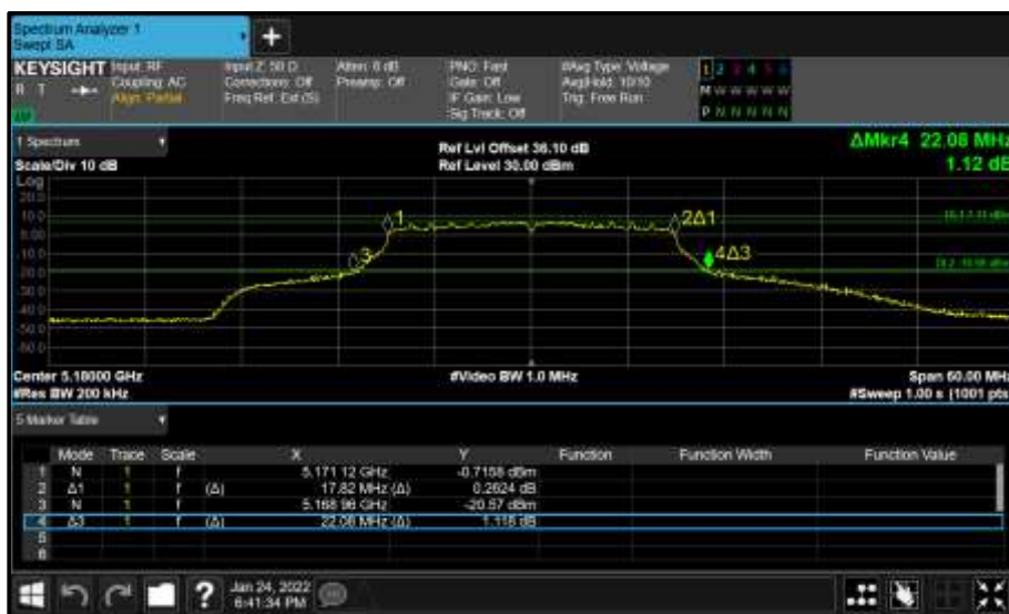
Figure 110 - Core 1 (B) 5180 MHz (CH36) 26 dB and 99% Bandwidth
