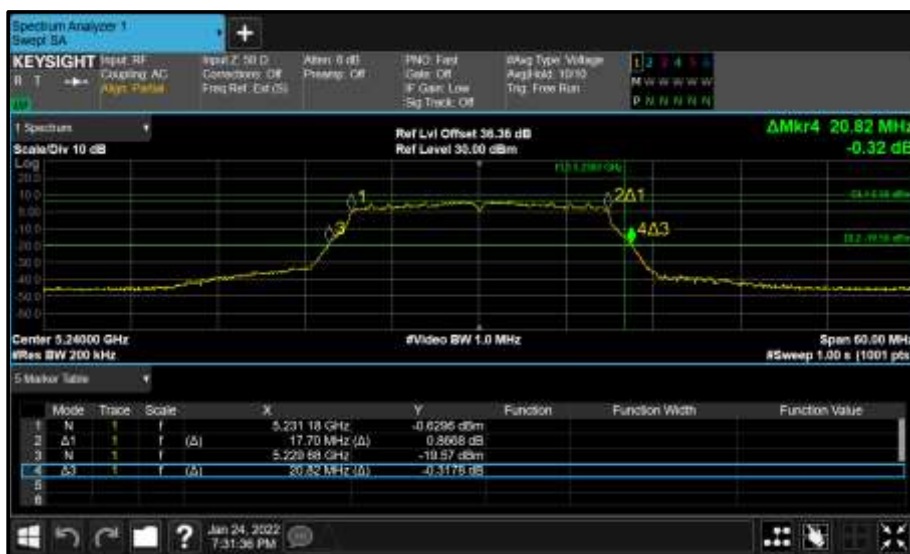
Figure 120 - Core 1 (B) 5240 MHz (CH48) 26 dB and 99% Bandwidth
