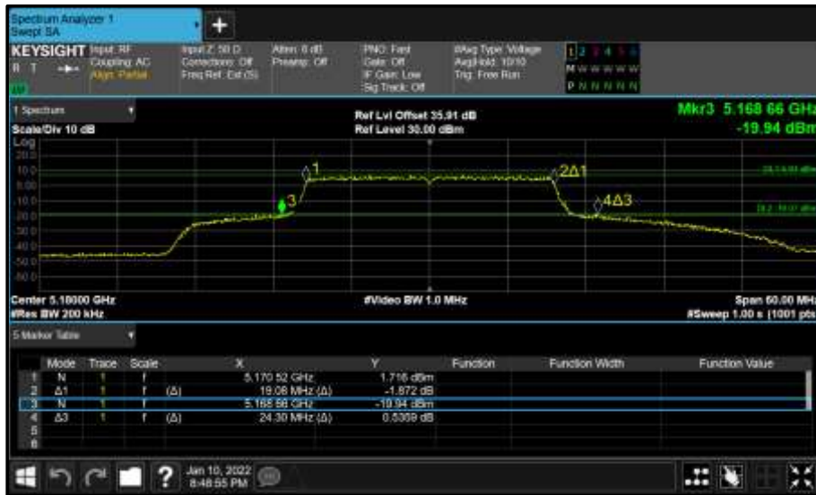
Figure 154 - Core 0 (A) 5180 MHz (CH36) 26 dB and 99% Bandwidth
