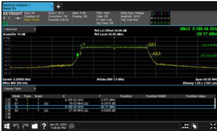
Figure 177 - Core 0 (A) 5200 MHz (CH40) 26 dB and 99% Bandwidth
