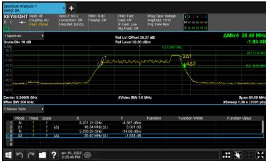
Figure 183 - Core 0 (A) 5240 MHz (CH48) 26 dB and 99% Bandwidth
