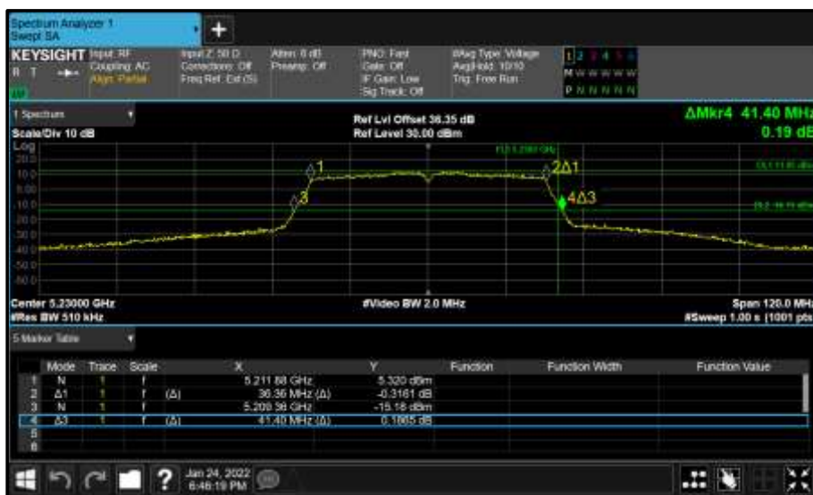
Figure 136 - Core 1 (B) 5230 MHz (CH46) 26 dB and 99% Bandwidth
