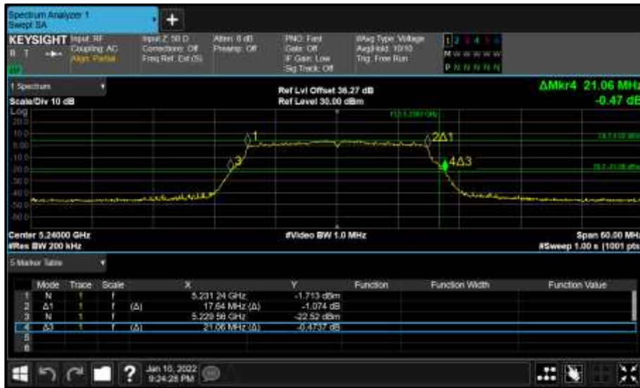
Figure 107 - Core 0 (A) 5240 MHz (CH48) 26 dB and 99% Bandwidth
