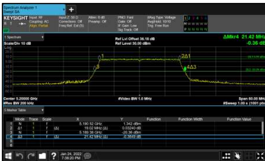
Figure 178 - Core 1 (B) 5200 MHz (CH40) 26 dB and 99% Bandwidth
