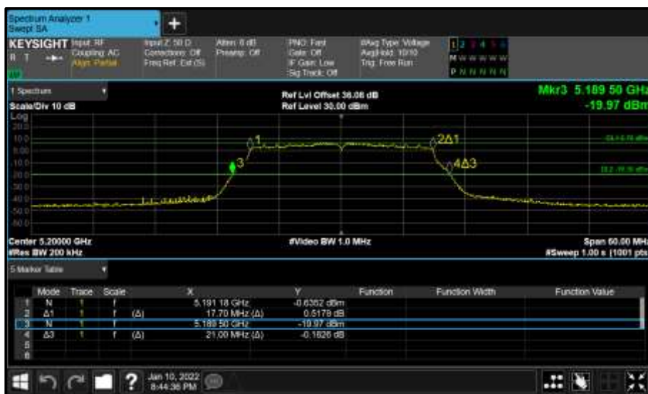
Figure 95 - Core 0 (A) 5200 MHz (CH40) 26 dB and 99% Bandwidth
