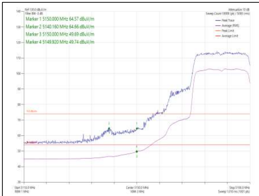
Figure 17 - 802.11ax HE20 SDM, Cores 0-1, SU - 5180 MHz Band Edge Frequency 5150 MHz
