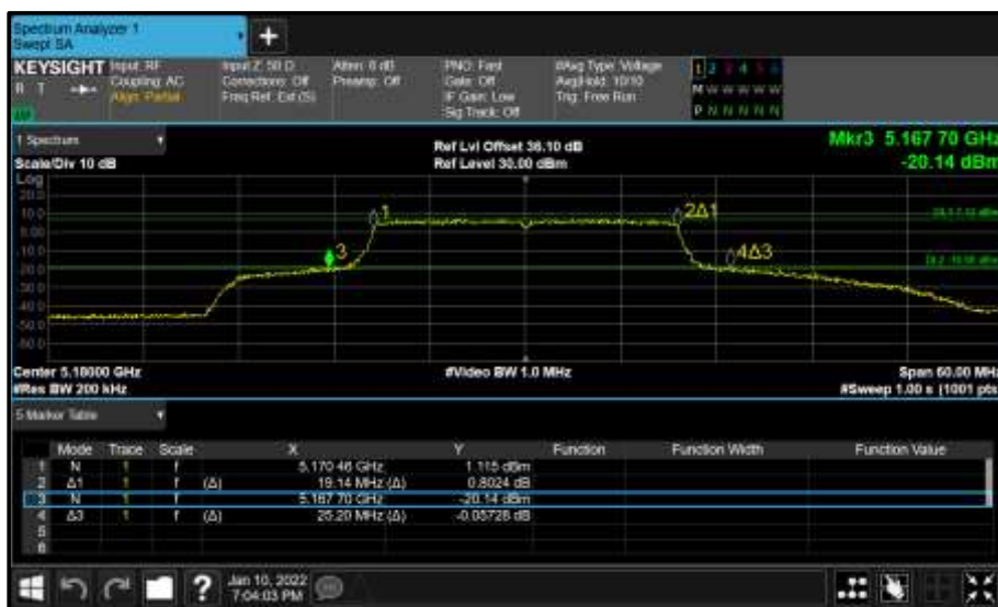
Figure 158 - Core 1 (B) 5180 MHz (CH36) 26 dB and 99% Bandwidth
