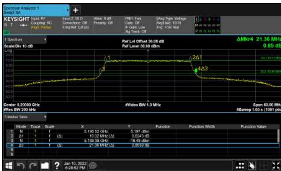
Figure 152 - Core 0 (A) 5200 MHz (CH40) 26 dB and 99% Bandwidth
