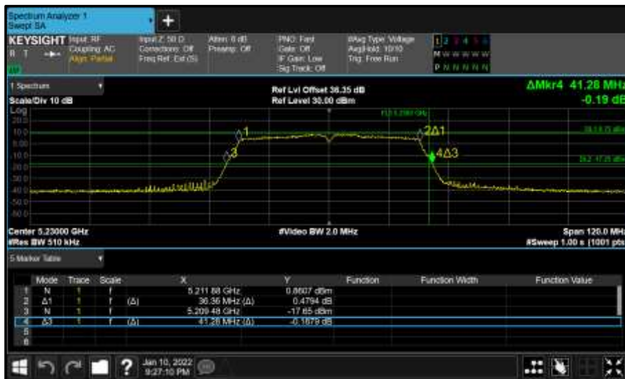
Figure 132 - Core 1 (B) 5230 MHz (CH46) 26 dB and 99% Bandwidth
