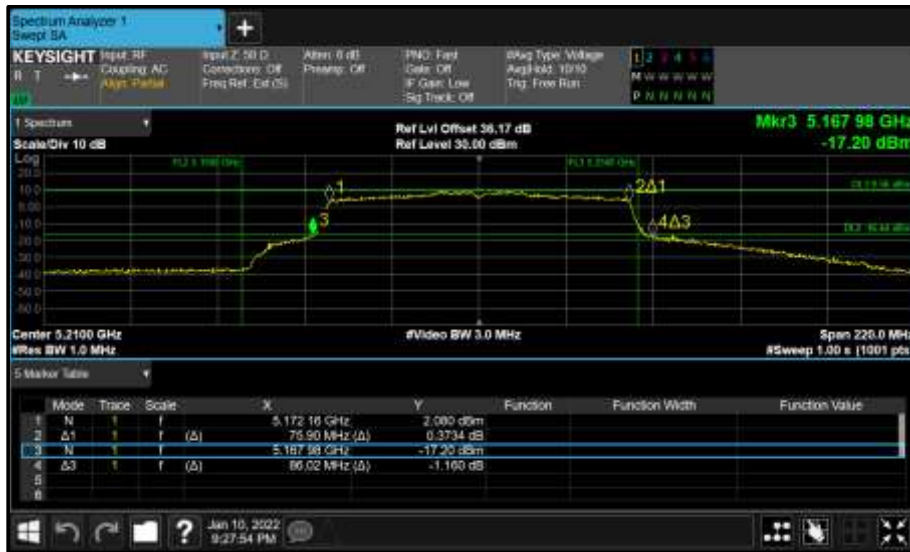
Figure 145 - Core 0 (A) 5210 MHz (CH42) 26 dB and 99% Bandwidth
