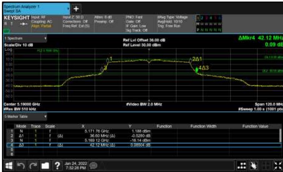
Figure 137 - Core 0 (A) 5190 MHz (CH38) 26 dB and 99% Bandwidth
