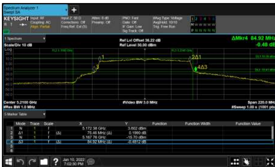
Figure 144 - Core 1 (B) 5210 MHz (CH42) 26 dB and 99% Bandwidth
