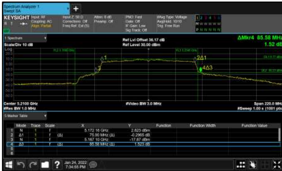
Figure 149 - Core 0 (A) 5210 MHz (CH42) 26 dB and 99% Bandwidth
