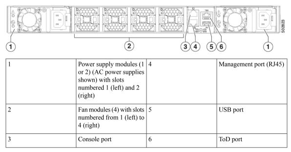
The following figure shows the side of the chassis.
