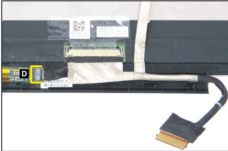
Figure 3-57. eDP Cable Removal
