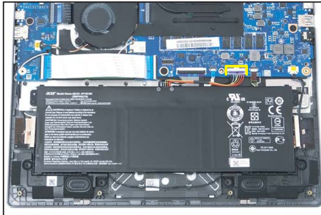
Figure 2-15. Battery Cable Disconnection
