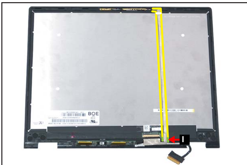
Figure 3-84. Replacing the eDP Cable
