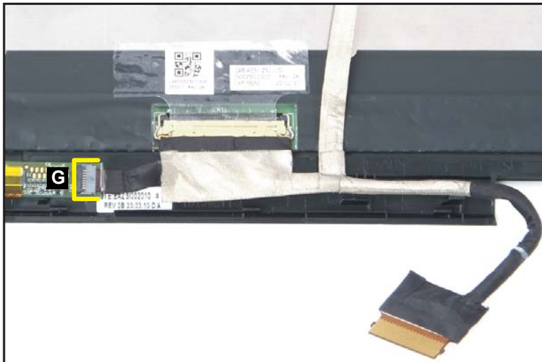
Figure 3-82. Replacing the eDP Cable
