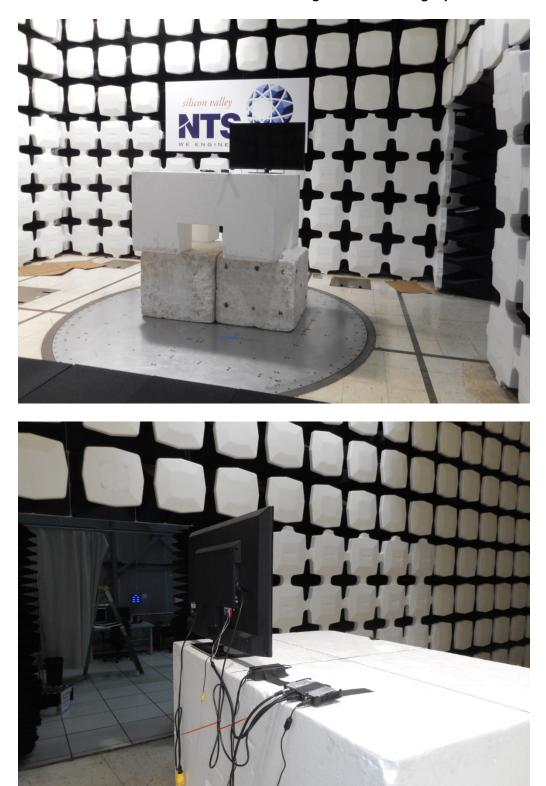
Radiated Emissions Test Configuration Photographs
