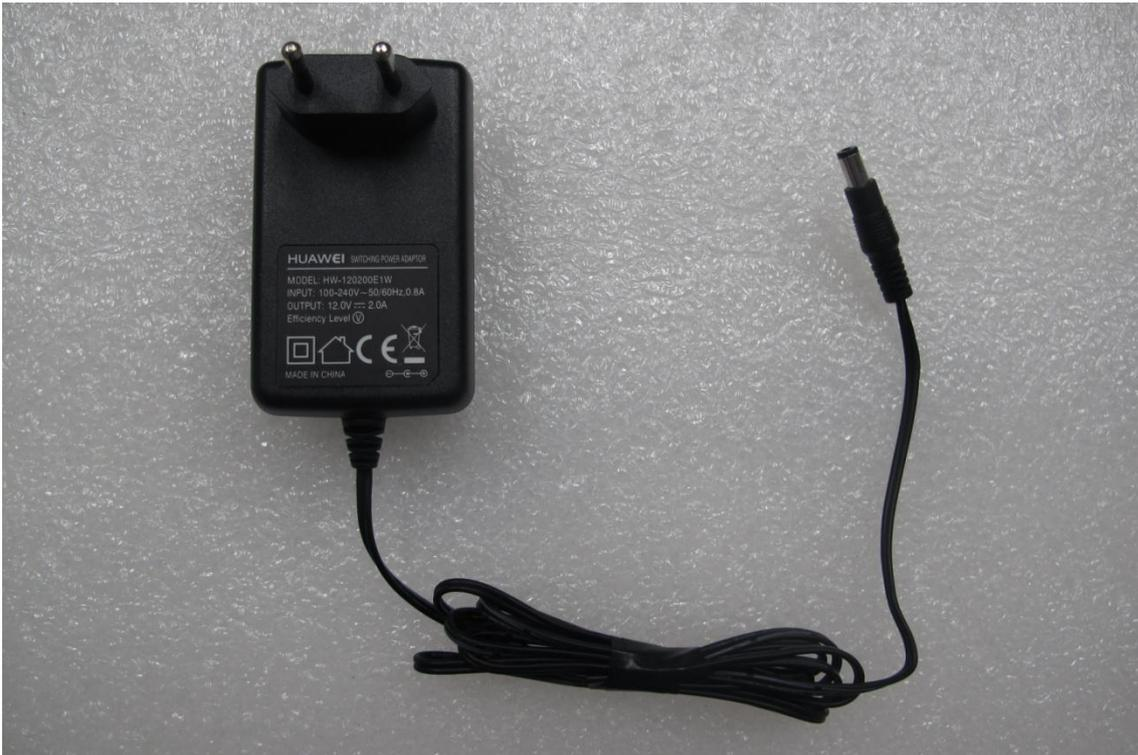
Figure 5. Adapter appearance (FUHUA HW-120200E1W)
