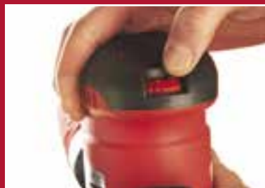
Variable speed selection (4000-10,000 rpm)
