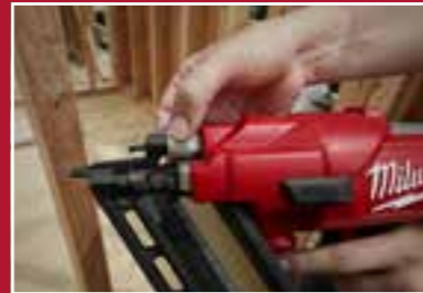
Tool-free, quick and easy depth adjustment
