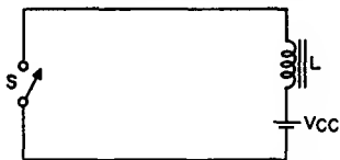
Fig. 85—Simplest form of deflection circuit.
