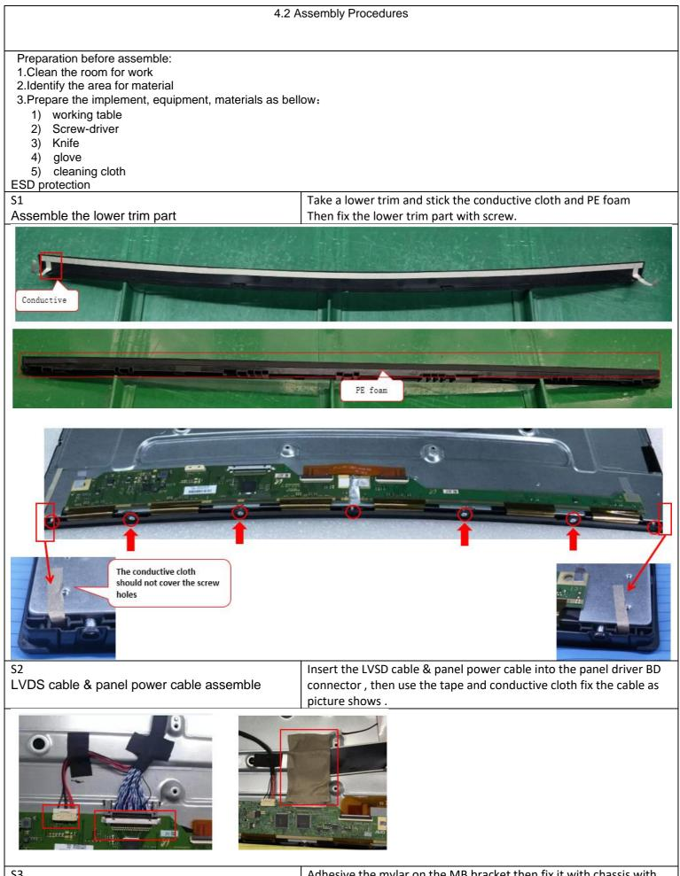
Assemble the MB and light bar power BD , and routing the cable
