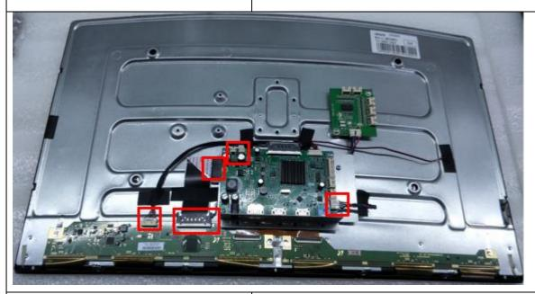
S4 Disassemble the MB, lamp power BD and MB bracket Unlock the screw and remove the MB & lamp power BD from the chassis bracket. Unlock the screw and disassemble the MB bracket from the chassis.
