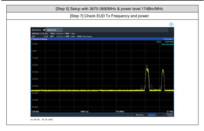
[Step 8.a.] After changing the frequency and power level, The module (EUT) discontinues operations, change frequencies, or change its operational power level within 10 seconds of receiving instructions from its associated CBSD. Test result is PASS.
