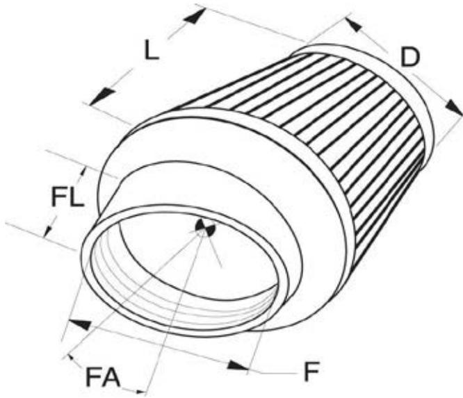
When selecting one of K&N's universal round tapered air filters, you should consider the following dimensions as they relate to the specification chart:
