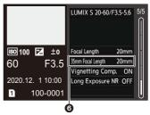
The focal length corresponding to the angle of view when using a full-frame lens with the [Aspect Ratio] set to [3:2]
