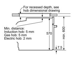
measurements in mm
